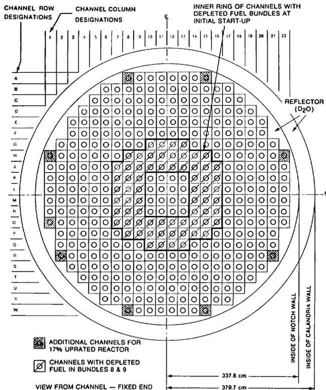
**FIGURE 1 END VIEW OF REACTOR SHOWING ADDITIONAL CHANNELS AND INNER RING OF 68 CHANNELS WITH DEPLETED FUEL**
