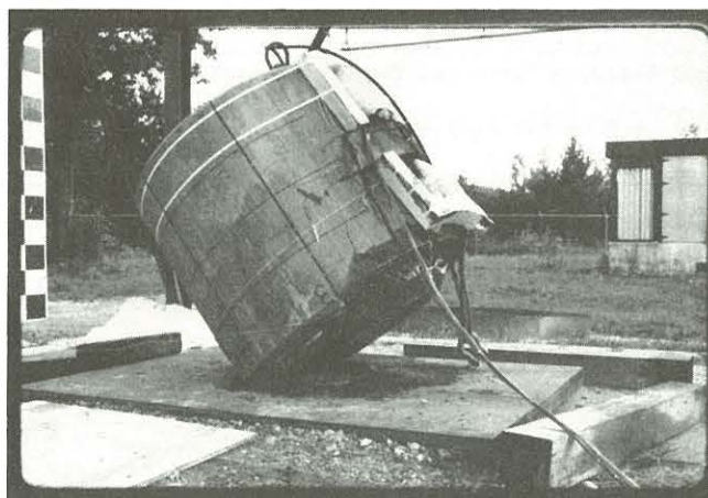
FIGURE 4: PIN DROP TEST
