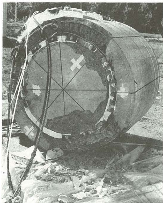
FIGURE 3: CASK MODEL AFTER 9 m DROP TEST
