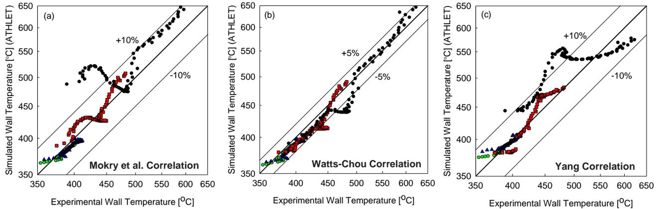
Figure 2: Error in Inside-wall Temperature for Low Mass Flux Cases (200 kg/m<sup>2</sup>s) using (a) Mokry et al. Correlation, (b) Watts-Chou Correlation, and (c) Yang Correlation
