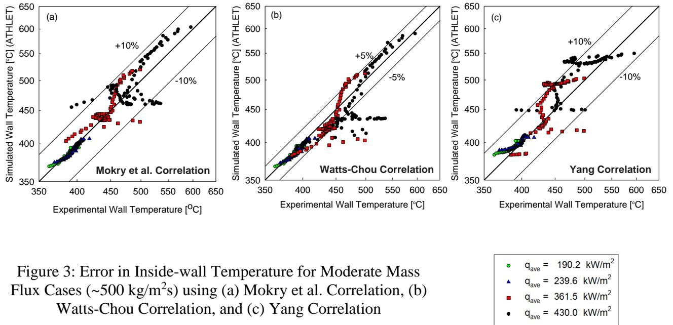
Figure 3: Error in Inside-wall Temperature for Moderate Mass Flux Cases ( $\sim 500 \text{ kg/m}^2\text{s}$ ) using (a) Mokry et al. Correlation, (b) Watts-Chou Correlation, and (c) Yang Correlation
