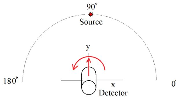
Figure 1 Schematic of point source and detector sweep arc in MATLAB program
