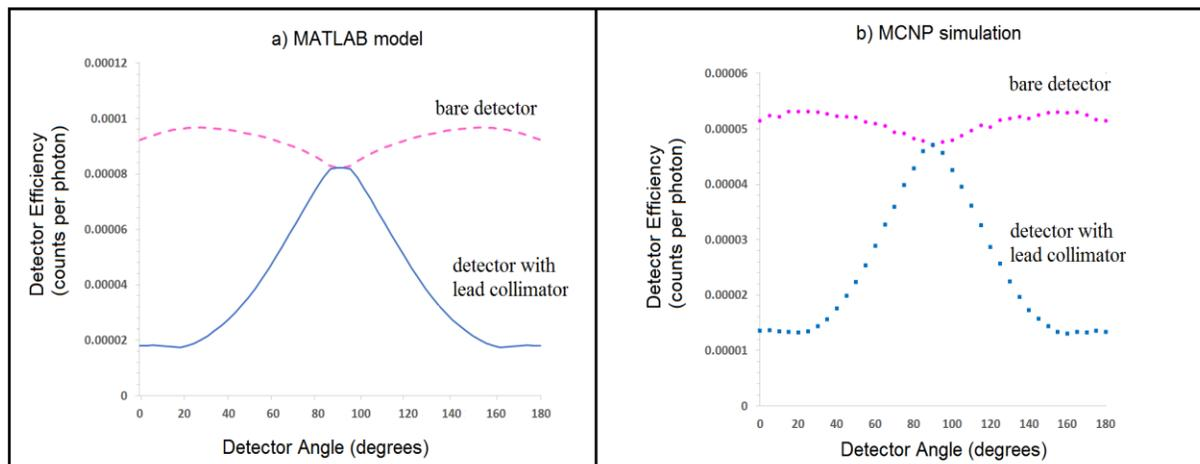
Figure 2 a) Output of MATLAB program for detector measuring point  $^{137}\text{Cs}$  source at 198 cm
