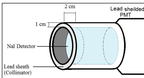
Figure 3 Schematic of NaI detector and lead collimator
