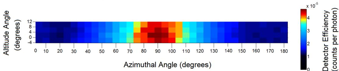
Figure 4 MCNP simulation for  $^{137}\text{Cs}$  point source at a distance of 198 cm and position  $(90^\circ, 0^\circ)$
