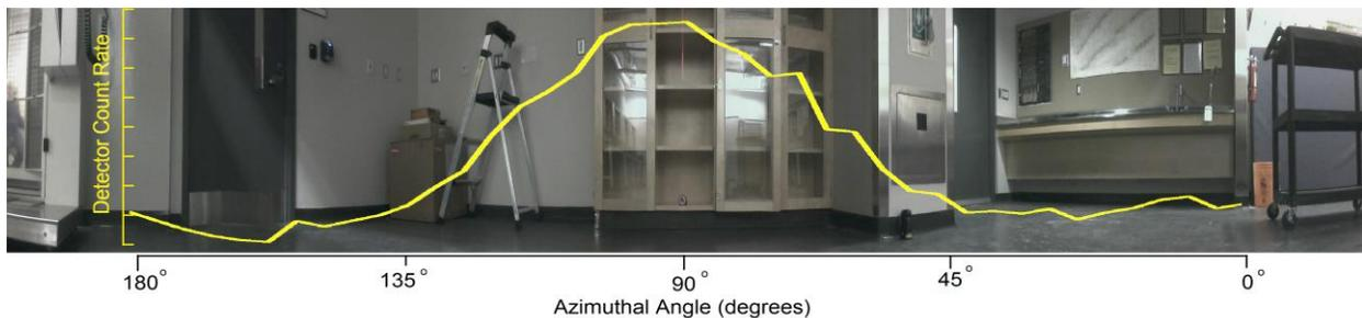
Figure 5 Visual panorama and overlaid gamma ray detector data from mobile robot
