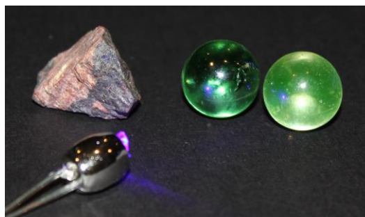
Figure 1: Image of samples FLTR: The Monazite crystal, a regular marble, a U-glass marble. Note the fluorescence in the U-marble caused by the blue light.
