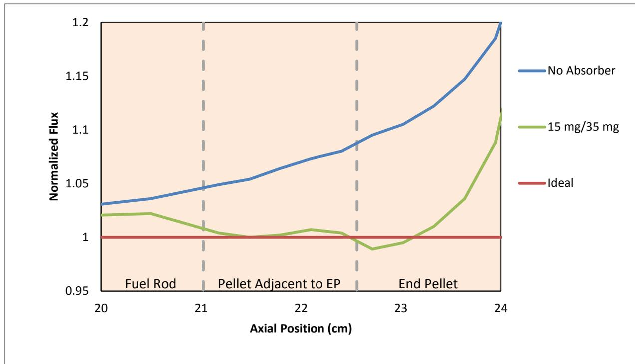
*Figure 2: Axial flux profile for the center element. For the absorber trial the first number represents the amount of absorber placed in the pellet adjacent to the end pellet and the second number is the amount of absorber placed in the end pellet*
