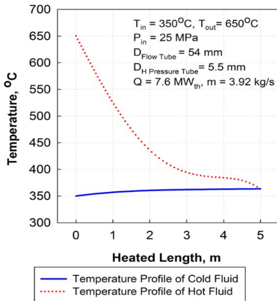
Figure 3: Temperature Profile along PCh.
