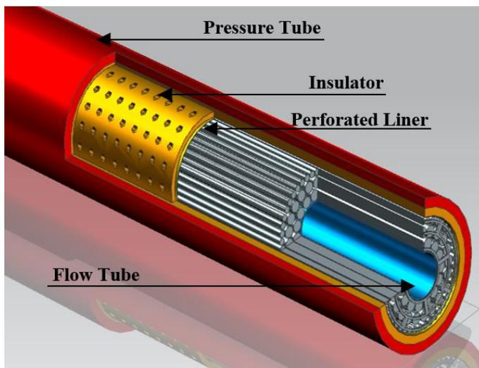
Figure 1: Re-entrant Channel Design
