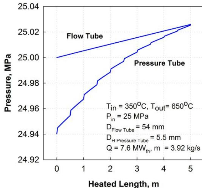
Figure 4: Pressure Profile along PCh.
