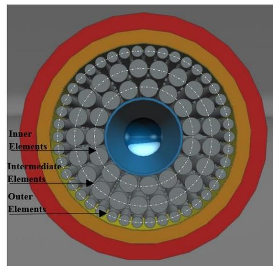
Figure 2: 78-element bundle cross section.
