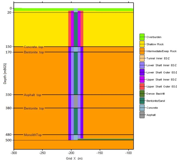
Figure 3: Ventilation Shaft Seal Design
