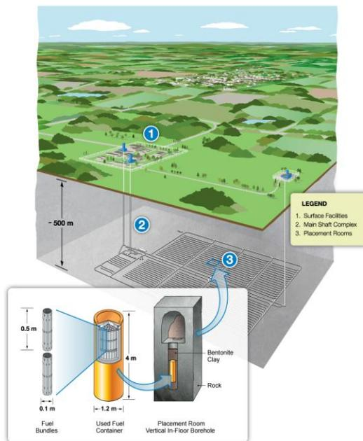
Figure 1: Conceptual Crystalline Rock Repository Design with IV-25 Containers
