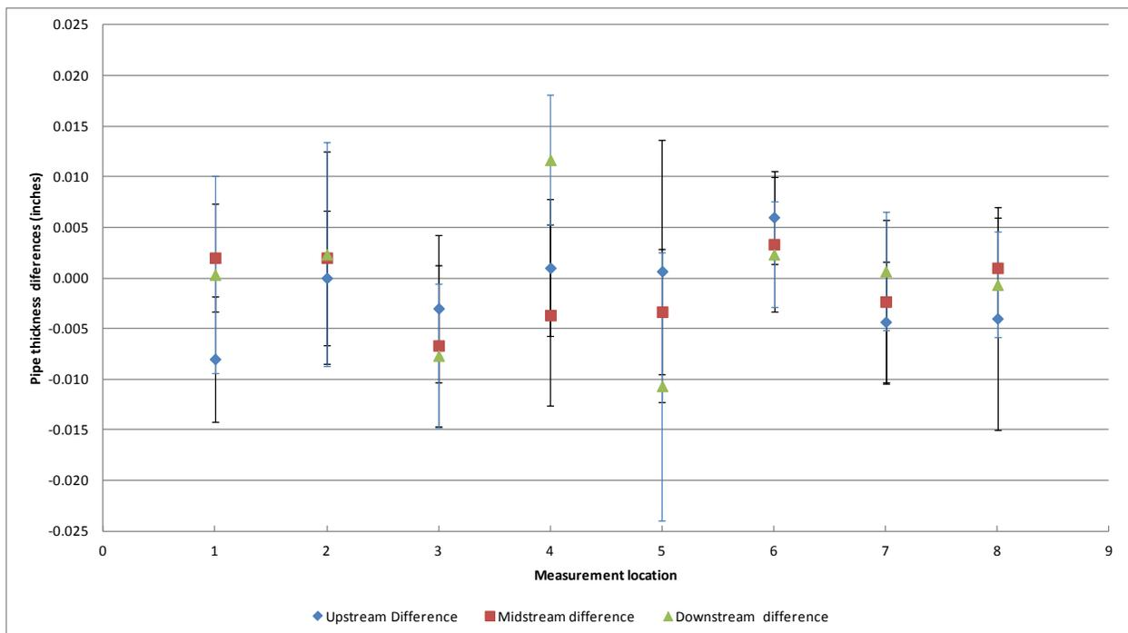
Figure 8 Difference in thickness measurement between teams A and B for Boiler 3
