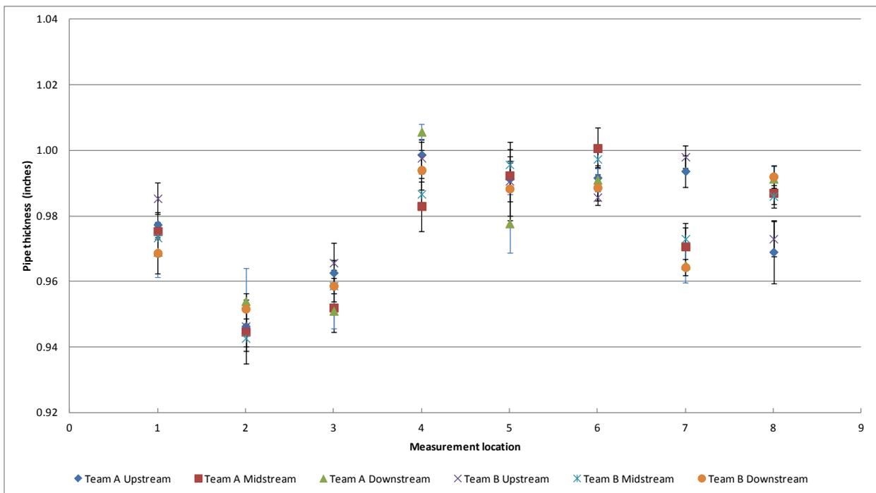
Figure 6 Point by point thickness measurement for Boiler 3
