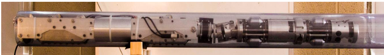
Figure 3: Robotic pipe crawler undergoing testing
