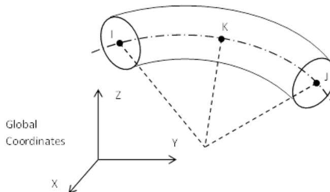
Figure 1 Illustration of ELBOW290 Element
