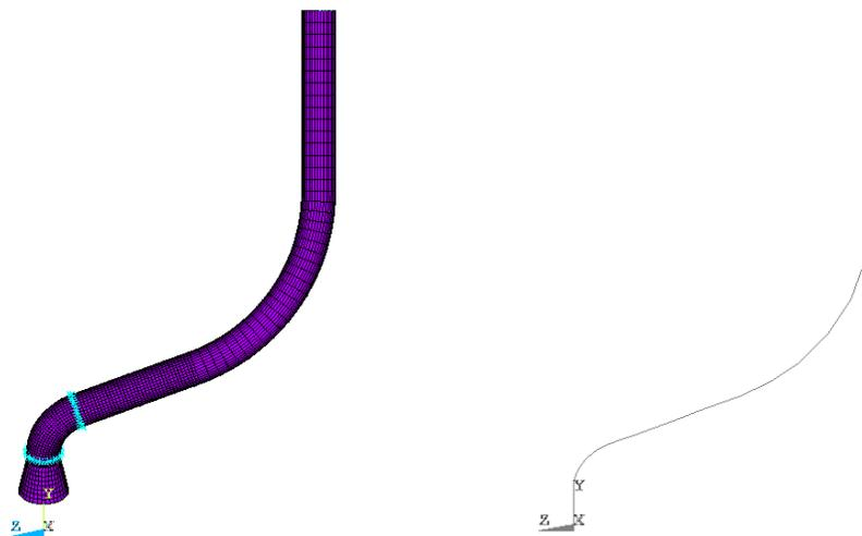
Figure 3 Representative Single Tight Radius Bend Modeled with Shell Elements (Left) and PIPE16/ELBOW290 Elements (Right)
