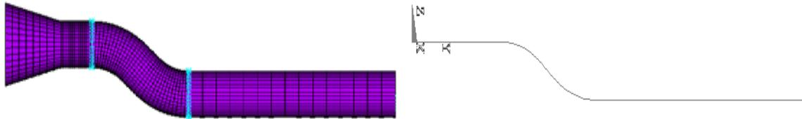
Figure 2 Representative Double Tight Radius Bend Modeled with Shell Elements (Left) and PIPE16/ELBOW290 Elements (Right)
