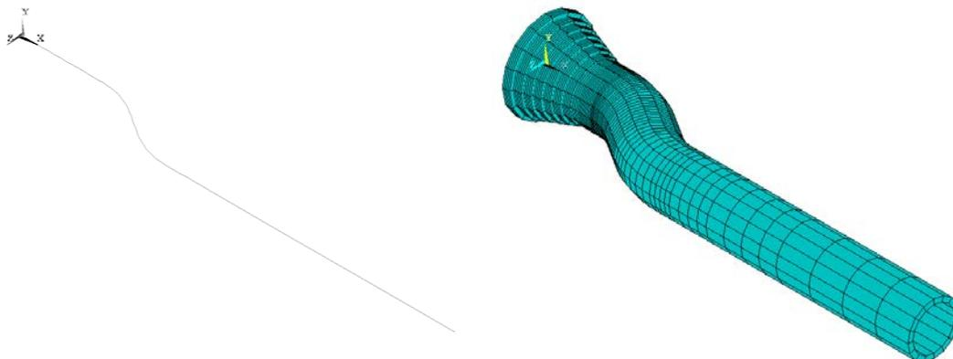
Figure 4 Typical Mesh of a Double Elbow with ELBOW290 elements: Plotted in Line Mode (Left);
