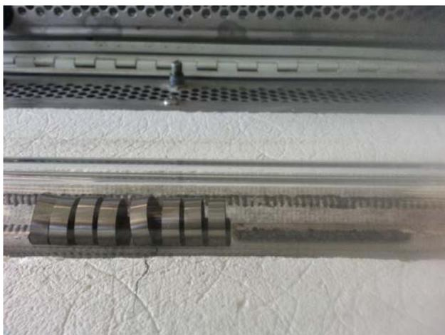
**Figure 1: Sealed capsule with ring-wedge assembly and iodine vial.**
