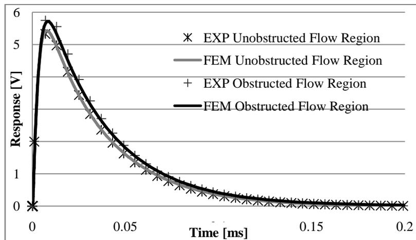
Figure 4 Experiment and FEM comparison of magnetite detection in broach support.
