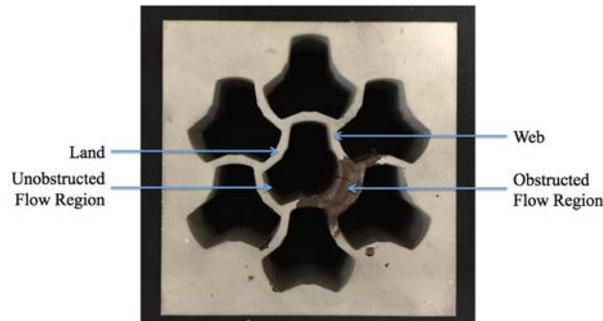
Figure 1 Sample broach support structure, exhibiting trefoil shape, with obstructed flow hole.
