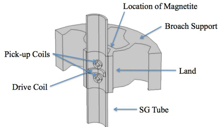
Figure 2 FEM one-third model for examining PEC response to magnetite in broach support structures.
