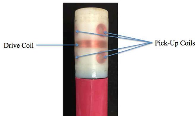
Figure 3 Experimental pulsed eddy current probe (only 4 of the 6 pick-up coils are visible).
