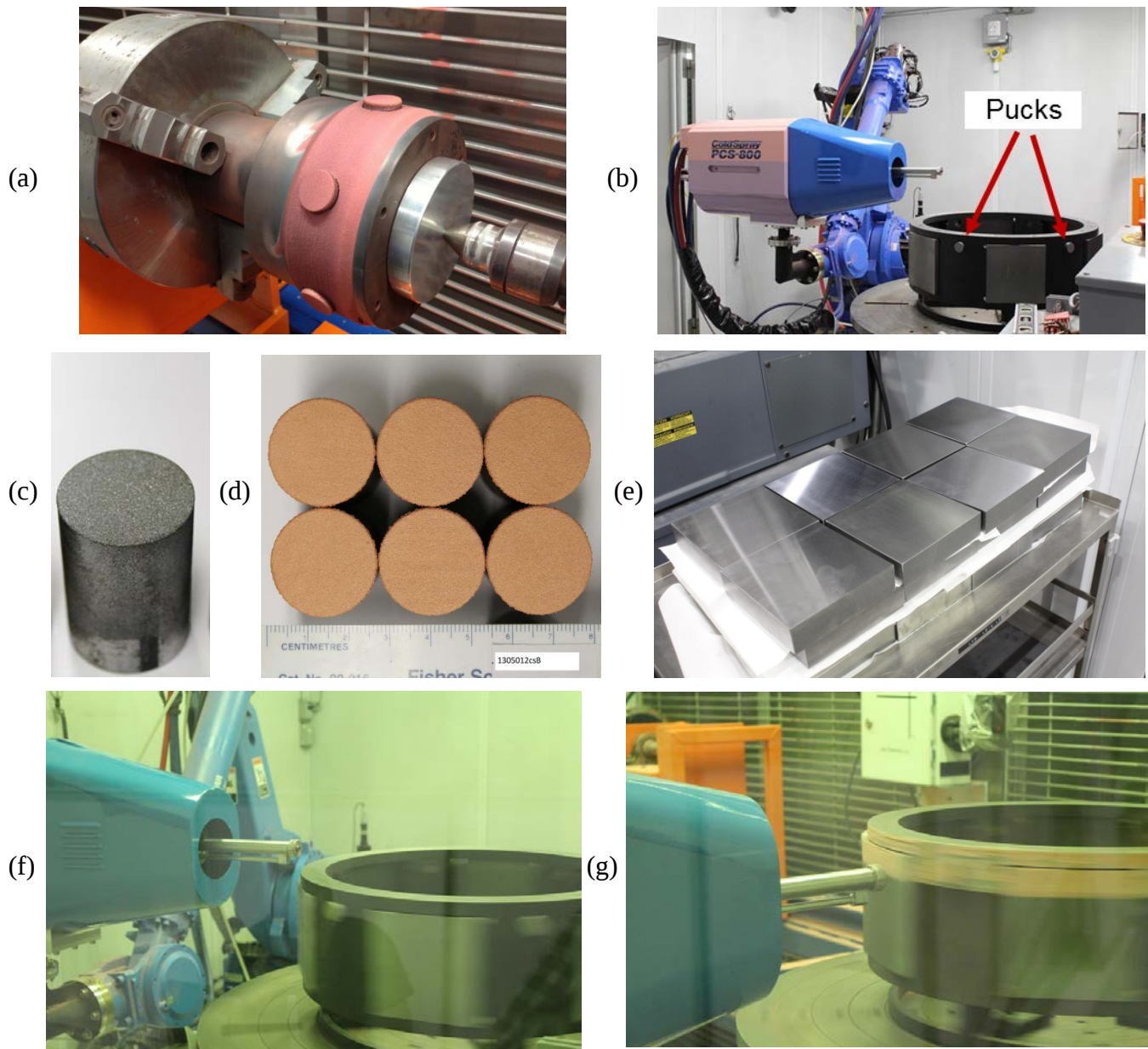
Figure 4: Cold Spray Development Components, including (a) Puck sample holder; (b) Plate and Puck holder; (c) Steel puck substrate (d) Coated puck samples (e) Steel Plates (f) Process at beginning and (g) Shortly after initiation of Cold Spray Coating.
