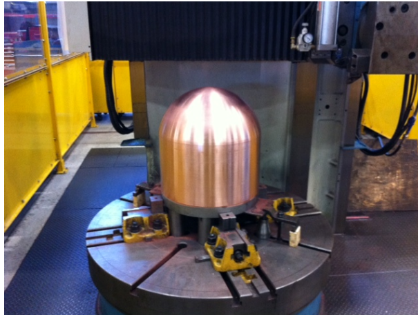
Figure 11: Coated and machined subsized container representing a full diameter lower section of the canister (i.e., full size hemispherical head and weld transition) with a truncated cylindrical body (560 mm Ø × 620 mm part length)
