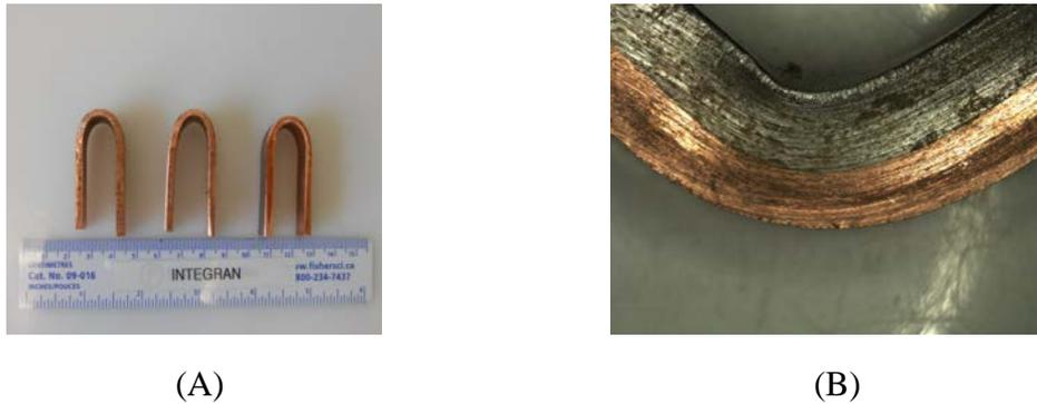
Figure 2: Electrodeposited copper bend test coupons showing (a) freestanding copper and (b) copper plated on steel
