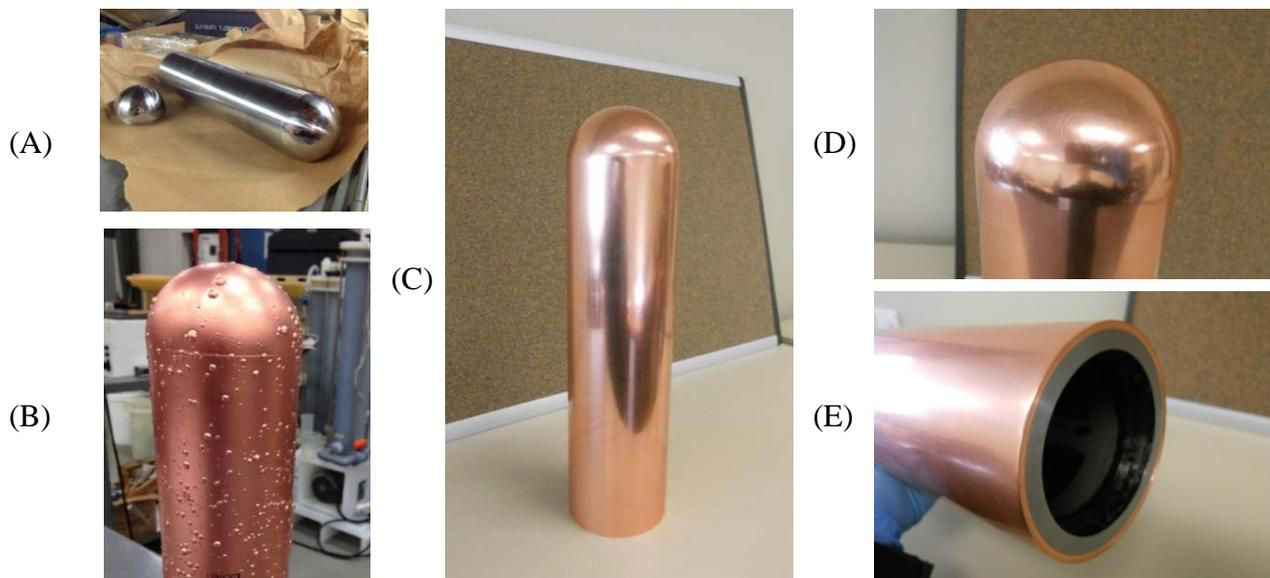
Figure 6: Images of small cylinder - 4"OD x 0.3" Wall x 12" Length – (A) uncoated with hemihead; and after application of copper to a target thickness of 3 mm: (b) as-deposited; as-machined showing (c) the full length; (d) the hemispherical portion and (e) the base.
