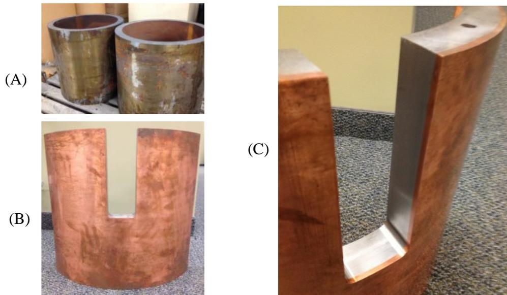
Figure 5 Images of 20" NPS schedule 120 pipe (A) as-received; and after application of copper to a target thickness of 3 mm to an arc segment 46 cm x 46 cm projection (b) facing view and (c) cross-sectional view (right).
