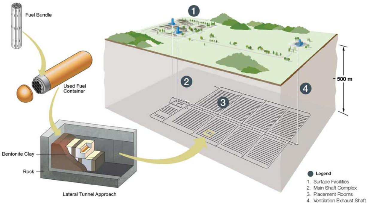
Figure 1: Schematic view of the deep geological repository concept for Mark II containers
