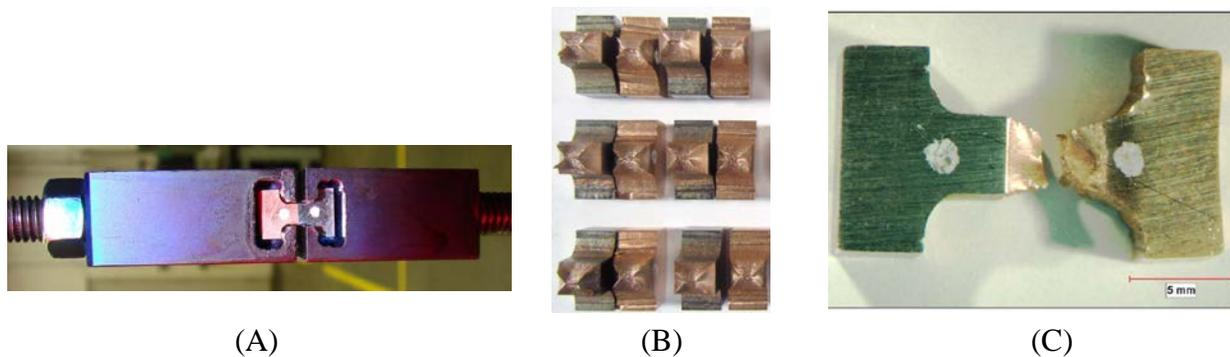
Figure 4: (A) Bi-metallic (copper-steel) E08 coupon for adhesion test in test rig and typical adhesion results (B) end-on view and (C) side-on view.
