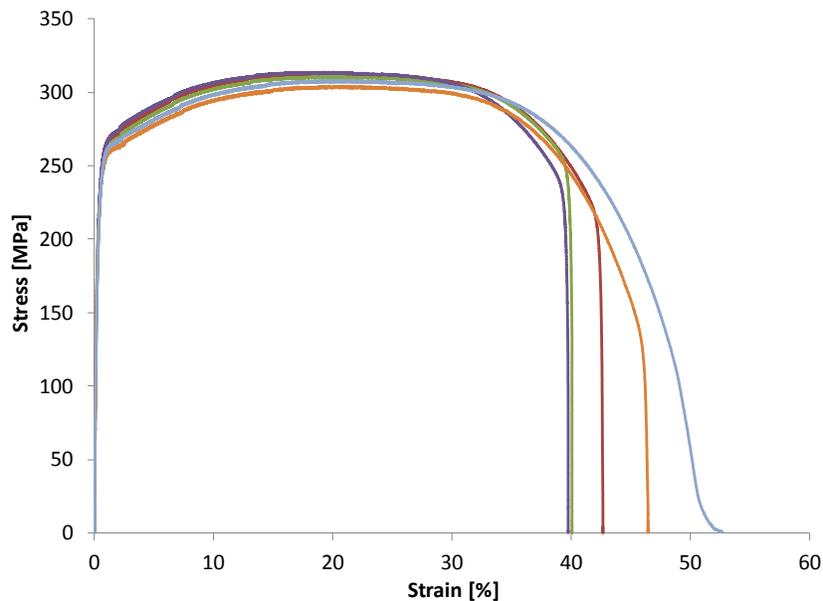
Figure 3 Electrodeposited copper coatings stress strain curves indicating high ductility (~40%) and high ultimate tensile strength (~300 MPa)
