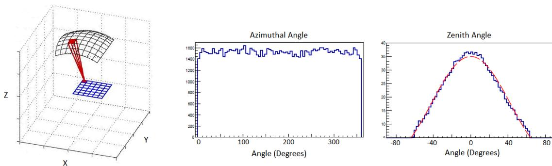
Figure 5 Left: Illustration of the division of muon events into angular bins. Horizontal muon detector shown in blue. A single angular bin has been highlighted in red. Middle and right: The angular distribution of muons at the surface of the earth.
