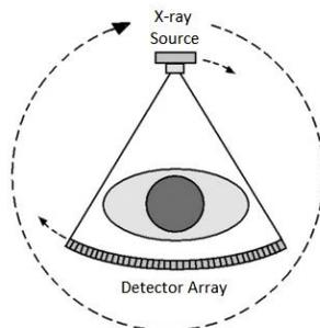
Figure 2 Schematic of the X-ray CT concept.
