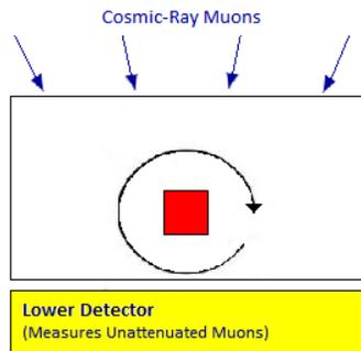
Figure 4 Object rotation within the CRIPT loading area to allow different detection points of view.
