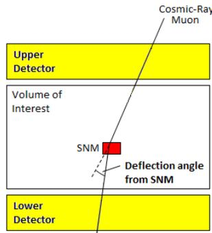
Figure 1 Schematic of the two-sided muon tomography concept.
