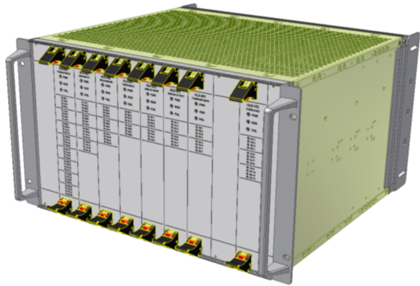
Figure 1 ALS Chassis Populated with Eight Boards.
