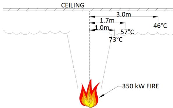
Figure 4 – Ceiling Jet Temperatures
