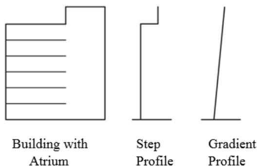
Figure 5 – Pre-fire room temperature profiles [2]
