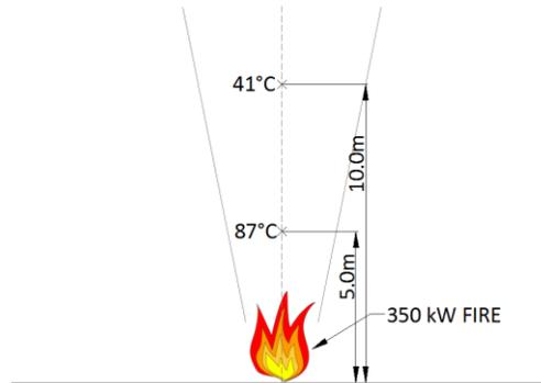
Figure 2 – Plume Temperatures
