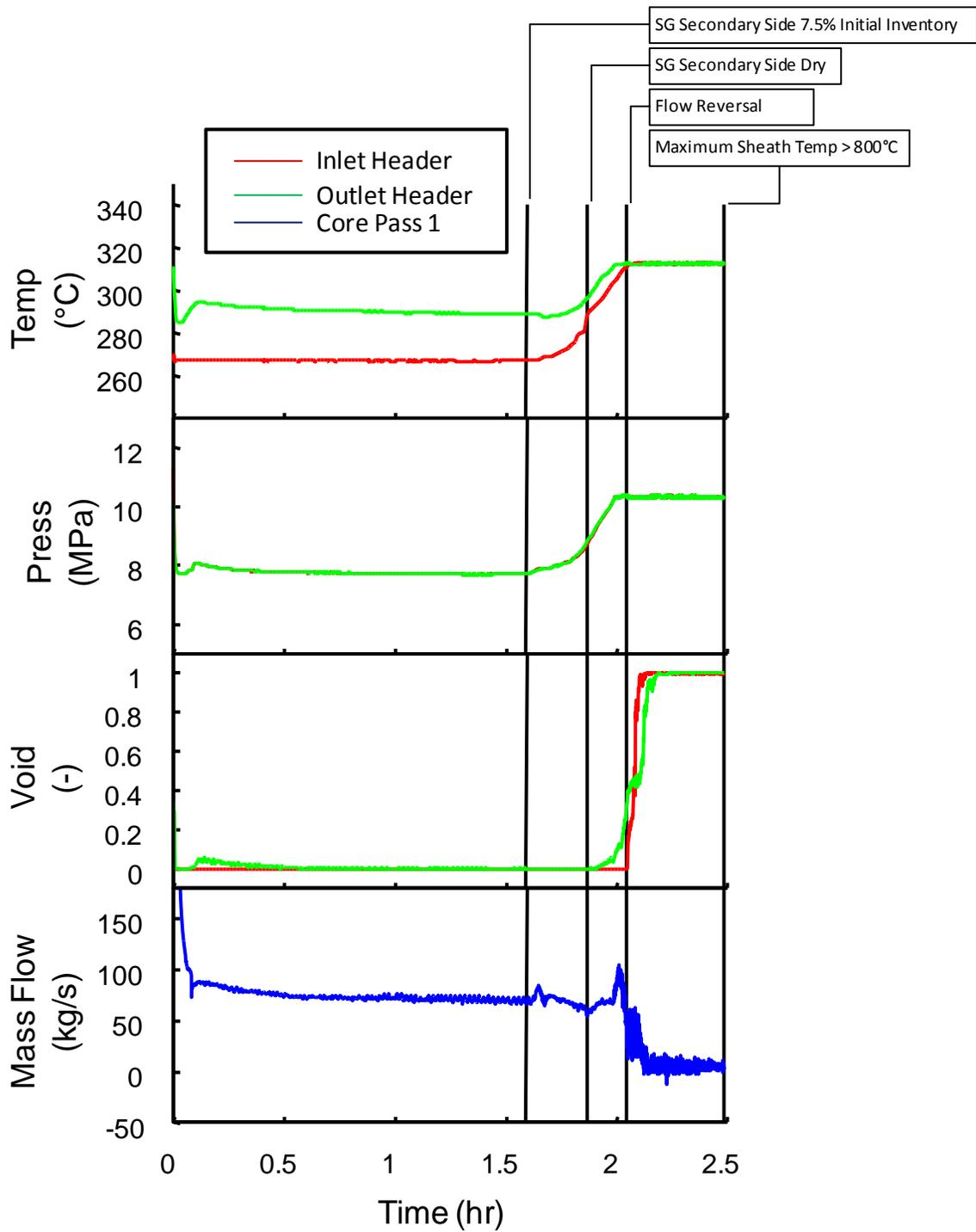
**Figure 4 Temperature, pressure, void, and mass flow rate for core pass 1. No crash cooling and high pressure ECC is unavailable.**
