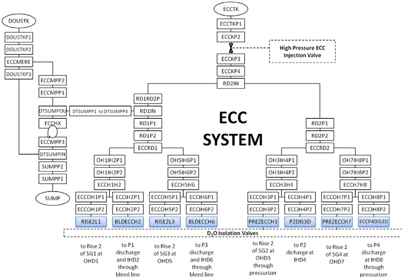
Figure 3 Flow diagram of CATHENA model (emergency core cooling system). Note that some details are omitted.
