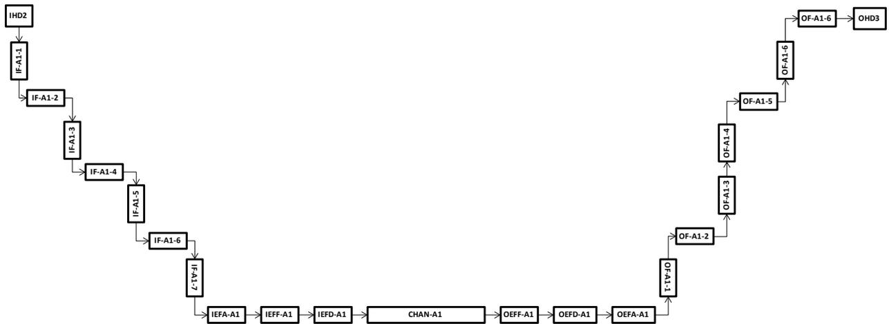
Figure 2 Flow diagram of CATHENA core model, core pass 1, channel group 1.
