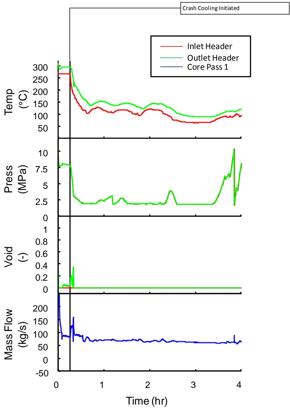
**Figure 7 Temperature, pressure, void, and mass flow rate for core pass 1. Crash cooling initiated 15 minutes after SBO and high pressure ECC is available.**
