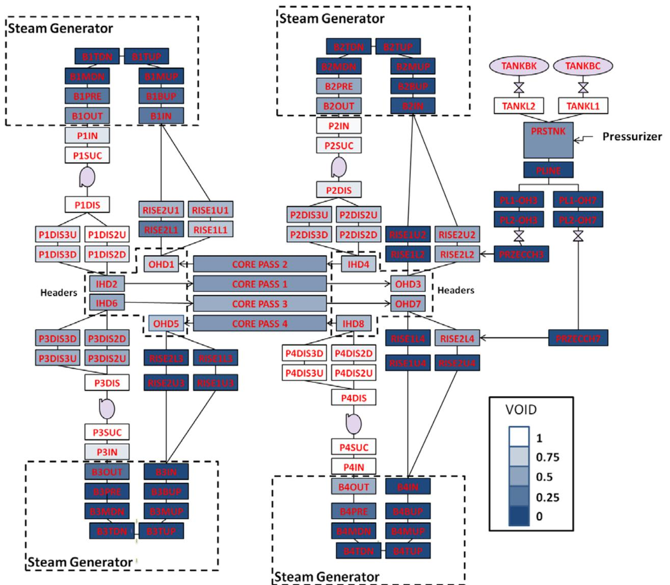
Figure 6 Void in the PHTS at 0.9 hr for scenario with crash cooling initiated 15 minutes after SBO and high pressure ECC unavailable.
