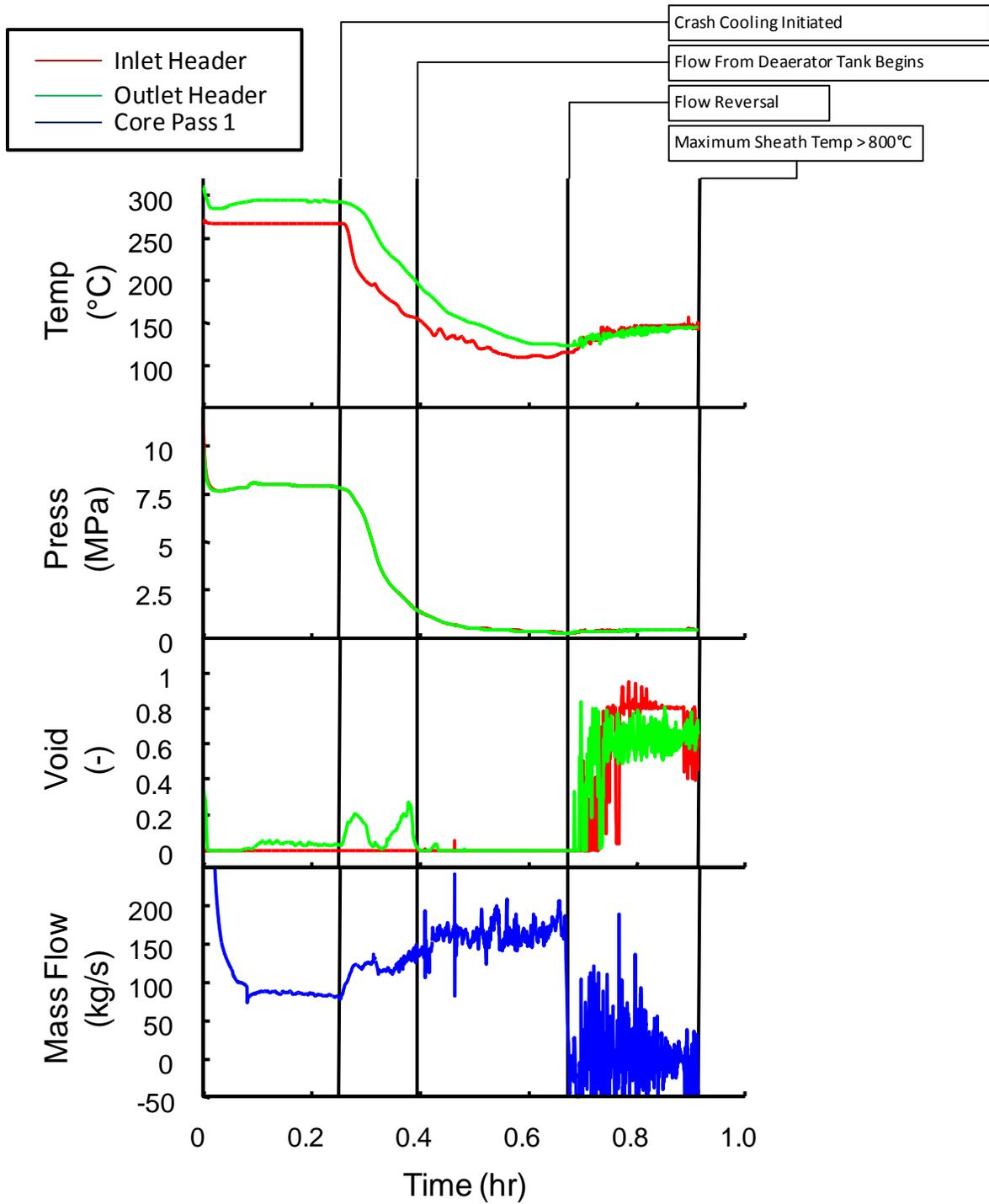
**Figure 5** Temperature, pressure, void, and mass flow rate for core pass 1. Crash cooling initiated 15 minutes after SBO and high pressure ECC is unavailable.
