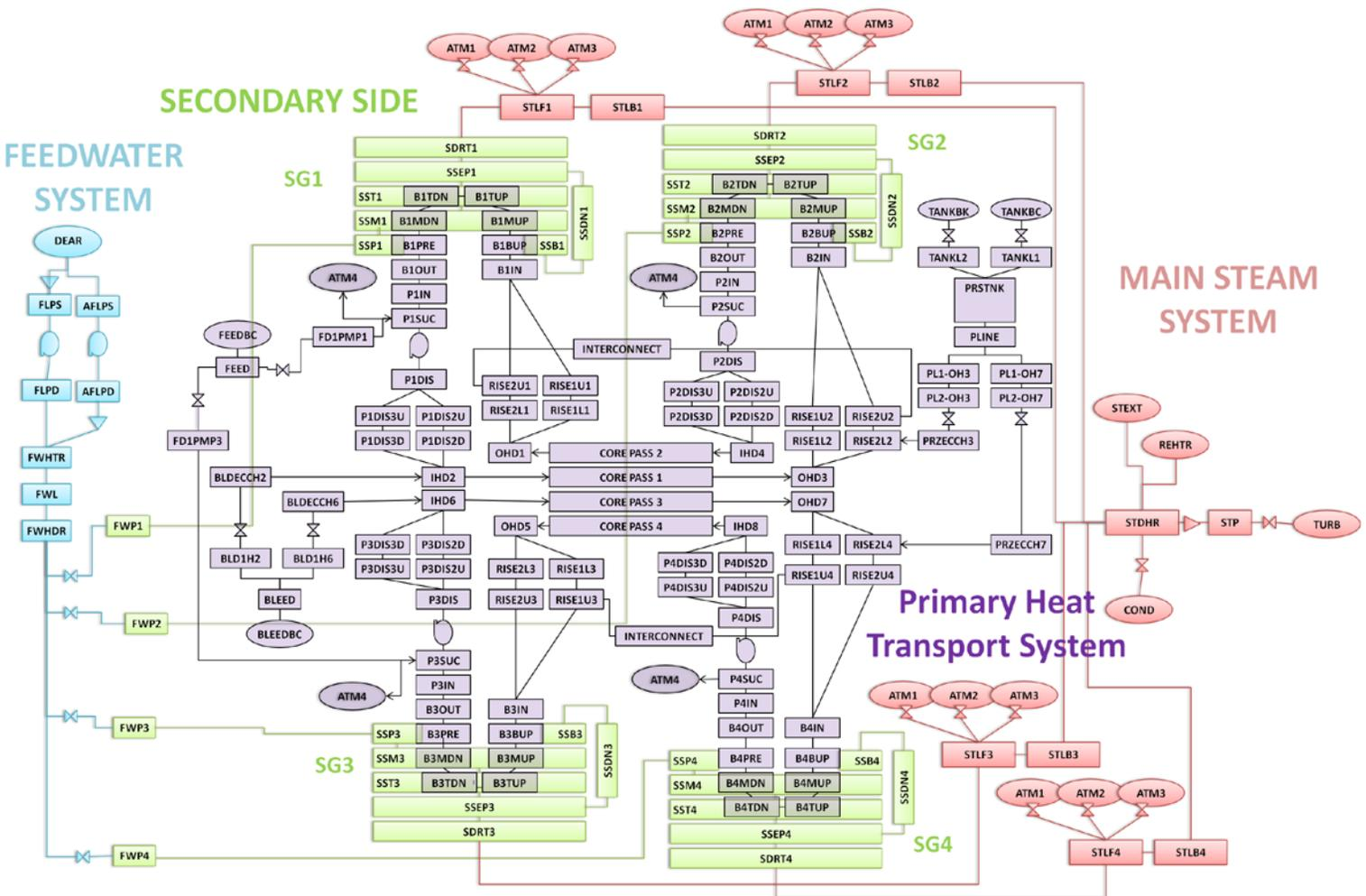
Figure 1 Flow diagram of CATHENA model (feedwater system, secondary side, main steam system, and primary heat transport system). Note that some details are omitted.
