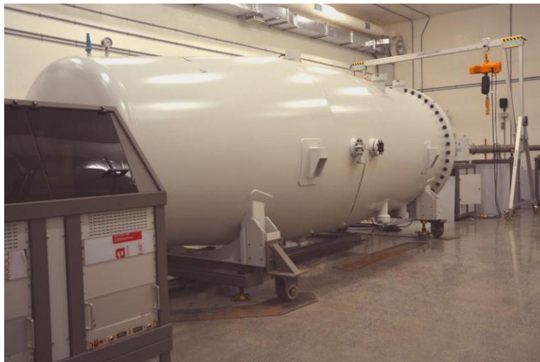
Figure 2. The High Voltage Engineering Europa 4MV Tandetron tandem accelerator at RMTL. The ion injector is partially visible at the left, one of the beam-tubes at the right.
