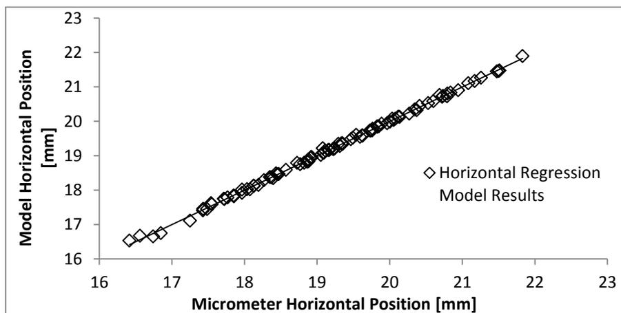
Figure 3 Horizontal tube position predicted by the regression model compared to horizontal micrometer measurements presented with best fit line through the data at 95 different locations.
