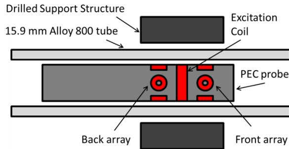
Figure 1 Schematic of the PEC probe inside an Alloy 800 SG tube and drilled support structure viewed horizontally. 4 of the vertically aligned coils can be seen side-on and 2 of the horizontal coils face-on.
