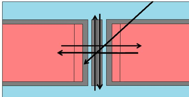
Figure 1: End Flux Peaking is created due to trapping of thermal neutrons, from all sources, in the end regions
