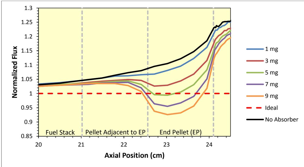
Figure 3: Preliminary absorber trials with various amounts gadolinium placed in the end pellet.
