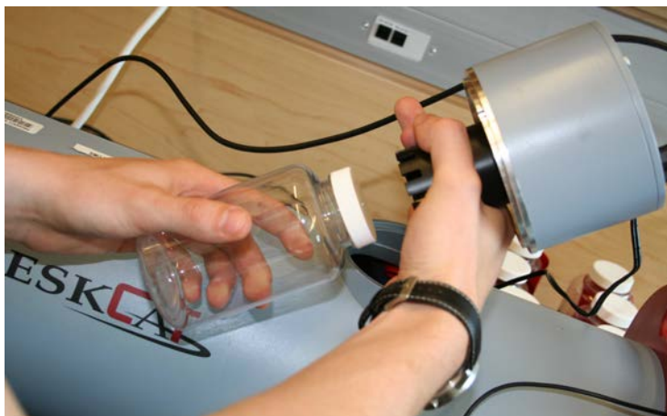
Figure Two: A sample jar being fit into the scanning head
