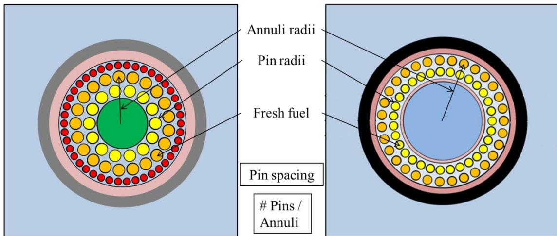
Figure 1: 78-Pin Fuel Assembly [5]
