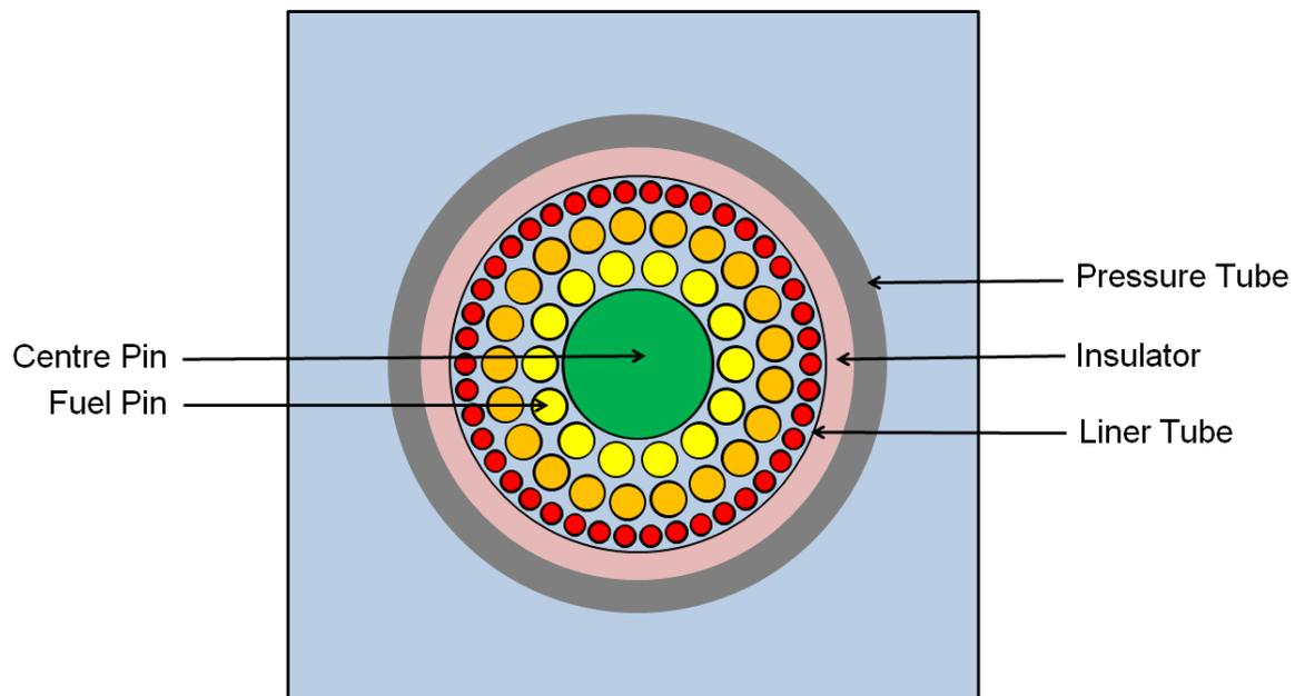
Figure 1 Cross-sectional view 77- element Canadian SCWR Fuel Assembly, with the element radii of the fueled elements being 0.68 cm for the two inner rings and 0.41 cm for the outer ring [2].
