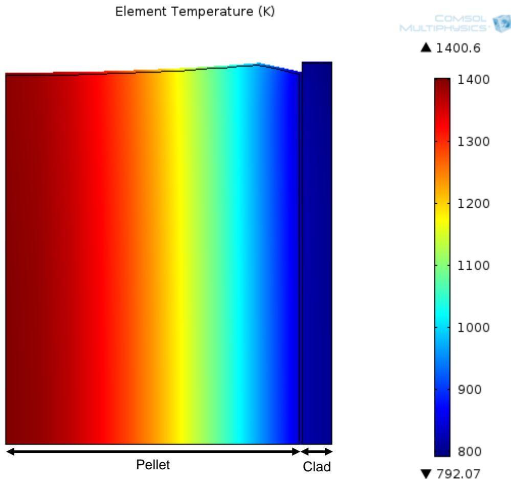
Figure 2 Temperature of an inner ring fuel element after 21 days irradiation with a LER of  $25 \text{ kW}\cdot\text{m}^{-1}$
