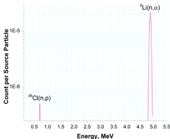
Figure 3: Detector Response Function to 0.1 MeV Neutrons
