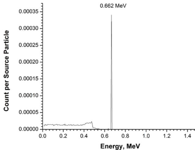
Figure 2: Detector Response Function to  $^{137}\text{Cs}$
