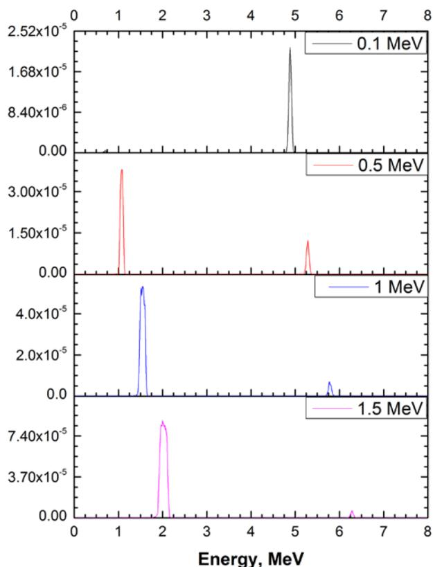
Figure 4: Detector Response Functions to 0.1 MeV, 0.5 MeV, 1 MeV, and 1.5 MeV Neutrons
