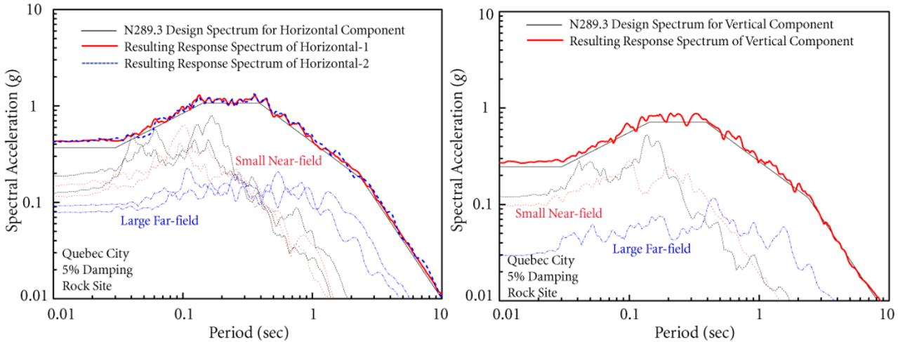
Figure 1 Resulting and target response spectra
