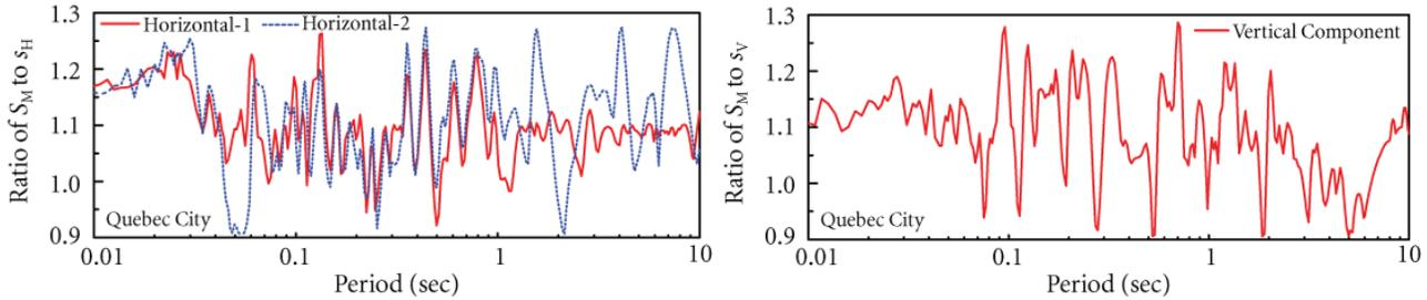
Figure 2 Errors between resulting and target response spectra.
