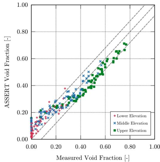
Figure 2: Accuracy of the ASSERT void fraction predictions for bundle B5 of the PSBT benchmark. Error bands represent the experimental error estimated at  $2\sigma = 0.08$ .
