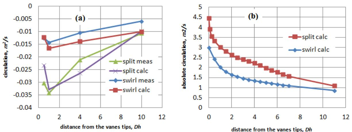
Figure 5: Decay of flow circulation downstream of mixing vanes a) circulation and b) absolute value of circulation.
