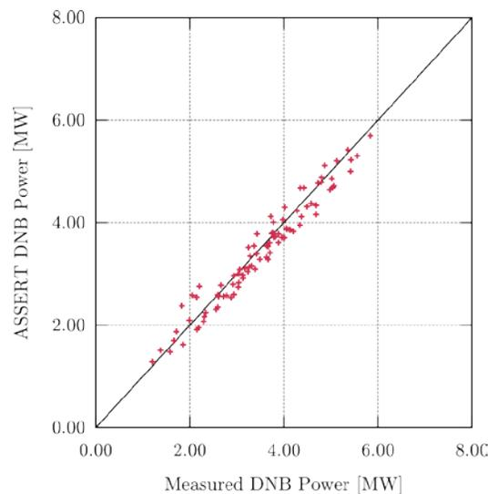
Figure 3: Accuracy of the ASSERT DNB Power predictions for test series A8 of the PSBT benchmark. Experimental uncertainty is estimated to be  $2\sigma = 2\%$ , and is not illustrated.
