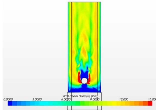
Figure 4: The unsteady flow behavior and turbulence generation around a single centralizing button within a PWR grid spacer.
