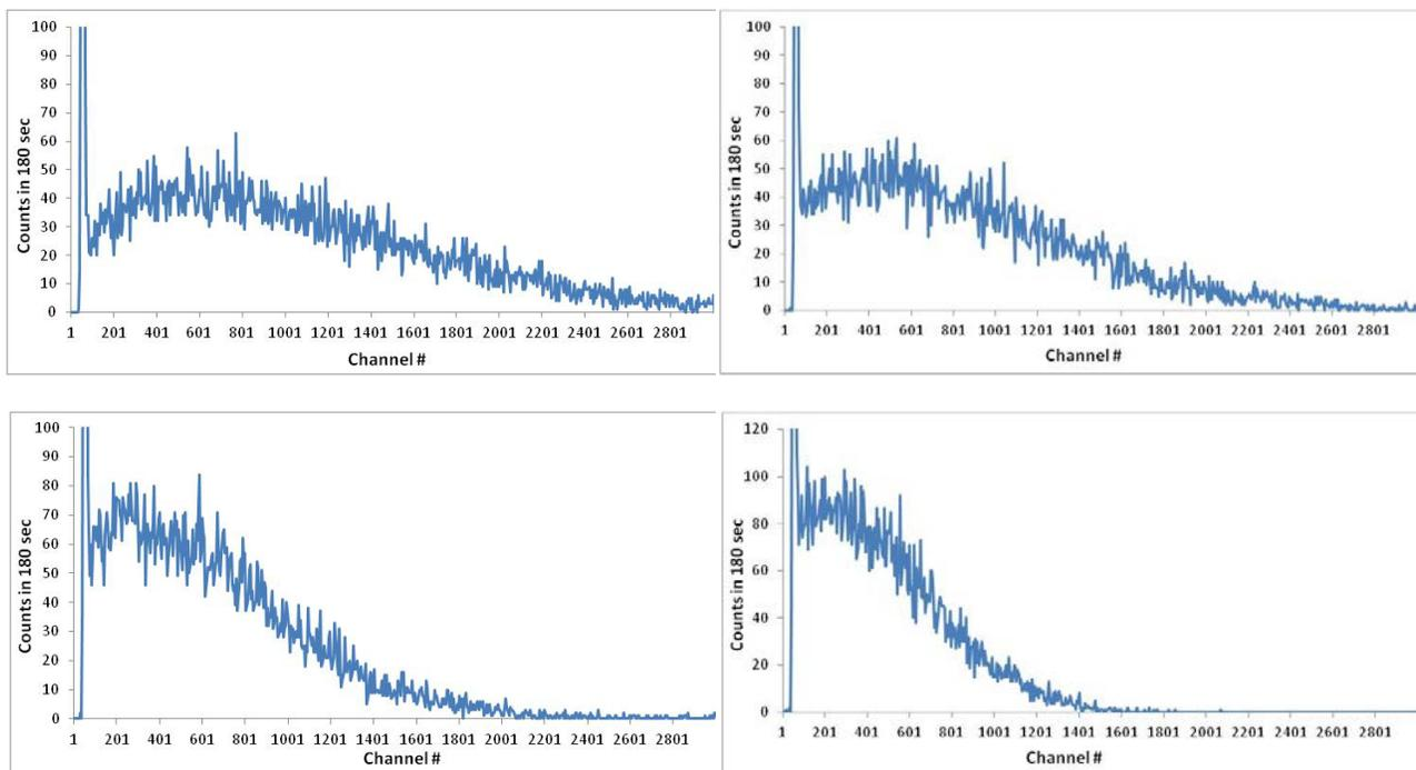
Figure 5 Pulse height spectrum of the ZnS[Ag] wet powder with Pu-239 source. a) very thin ZnS[Ag] powder; b) thin ZnS[Ag] powder; c) thick ZnS[Ag] powder; d) very thick ZnS[Ag] powder;
