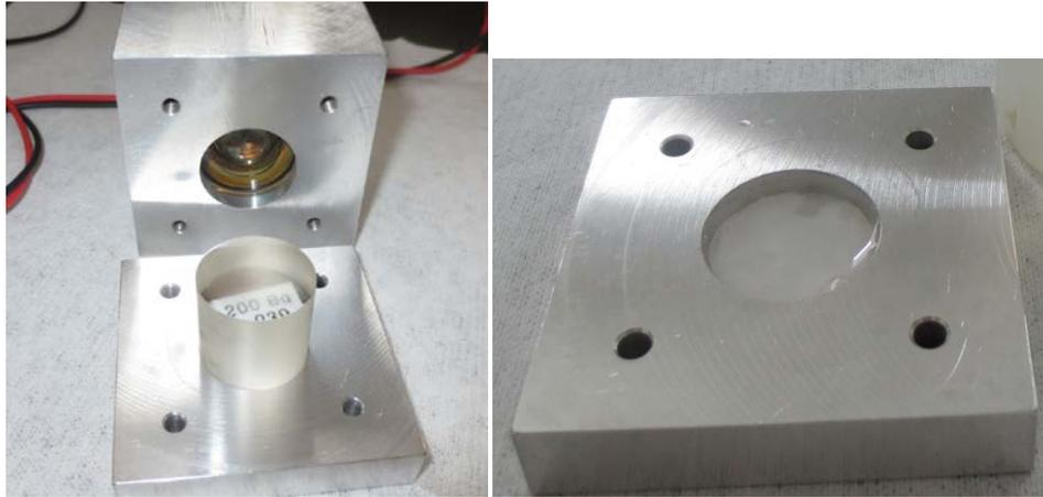
Figure 2 PMT and the Bottom Container with Pu-239 Source in the Container
