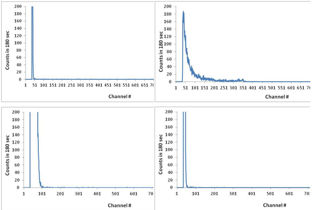
Figure 3 Background spectrum checks. a) Pu-239 source without scintillator; b) YAP[Ce] without Pu-239 source; c) ZnS[Ag] dry powder without source; d) ZnS[Ag] wet powder without source;
