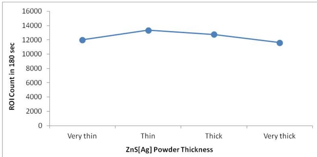
Figure 6 ROI counts vs. ZnS[Ag] powder thickness with Pu-239 alpha source
