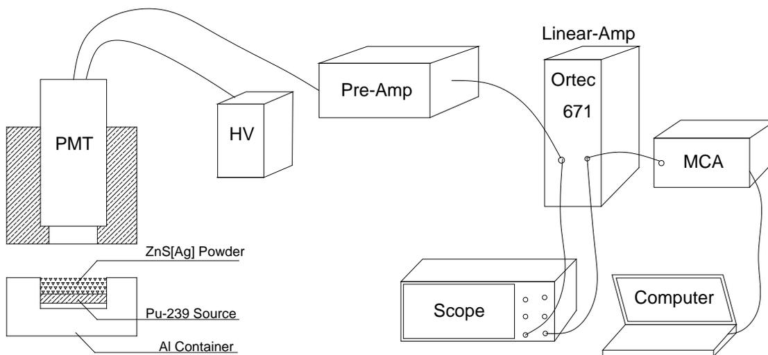
Figure 1 Block diagram of the experimental configuration for alpha detection
