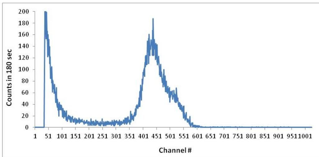
Figure 4 Pulse height spectrum from the YAP[Ce] with Pu-239 alpha source
