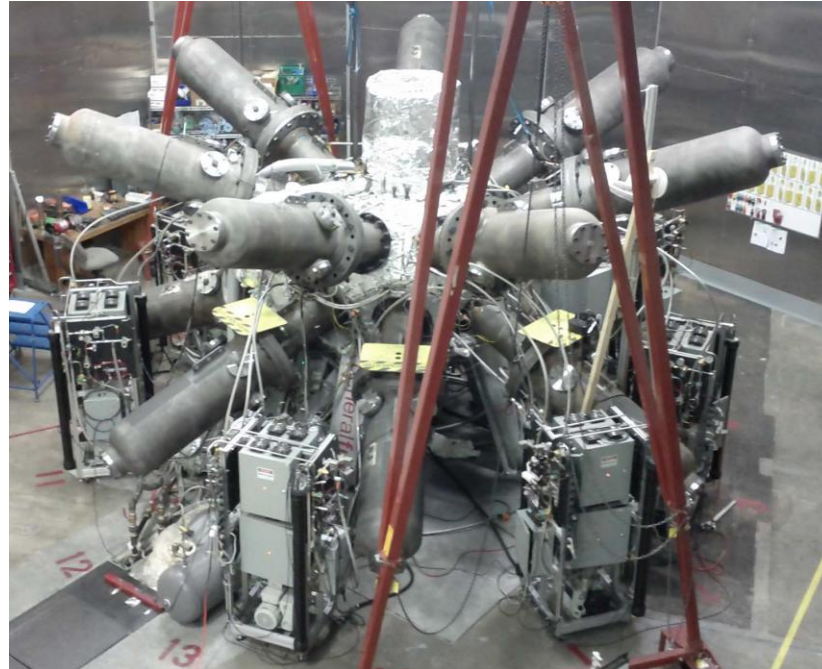
Figure 5: Mini-Sphere, a 1 meter spherical, liquid lead filled, tank with acoustic drivers mounted around the exterior, has 14 drivers, arranged in two rings of 7 drivers each. The hammers impact anvils that are in direct contact with the liquid lead, imparting pressure pulses into the molten metal. Lead is pumped around the inside of the sphere, creating a cylindrical vortex in the centre of the device. The inner wall of the vortex can then be imaged as pressure waves, travelling in from the radial pistons, converge and collapse the vortex
