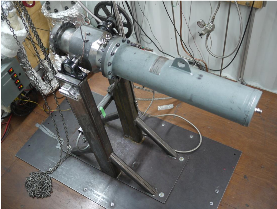
Figure 3: Mini-piston, in horizontal position, without lead tank installed. This machine, which is a 1/3 rd scale version of General Fusion's full scale pistons uses an air- actuated hammer in a bore that impacts a stationary anvil. A molten lead tank can be fitted onto this device to study both the pressure wave propagation in the liquid metal as well as the behavior of materials when they exposed to liquid metals under high loads.
