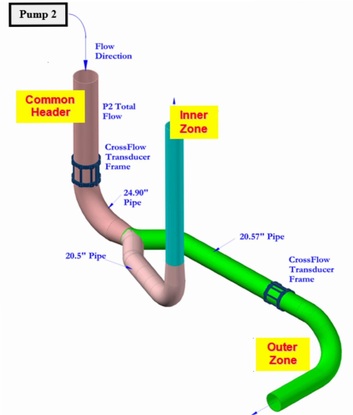
Figure 2 Bruce A Unit 1 Discharge Pump #2 piping configuration and installation locations
