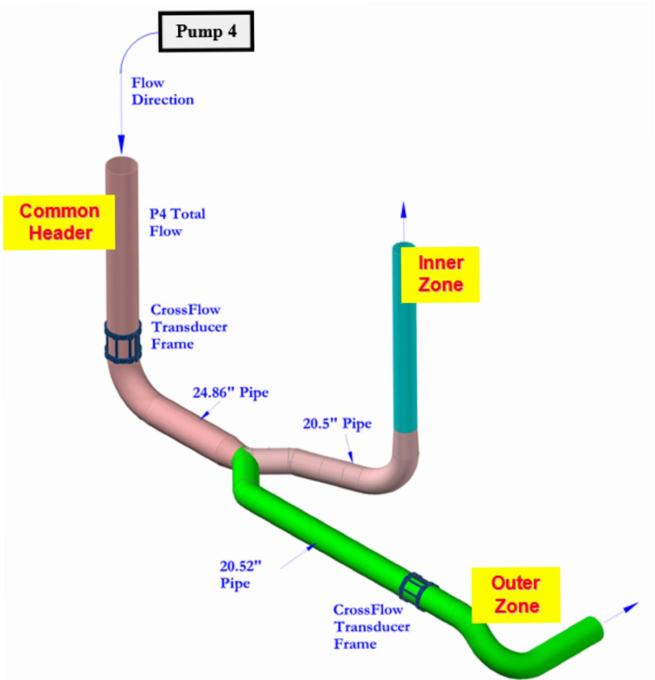
Figure 3 Bruce A Unit 1 Discharge Pump #4 piping configuration and installation locations
