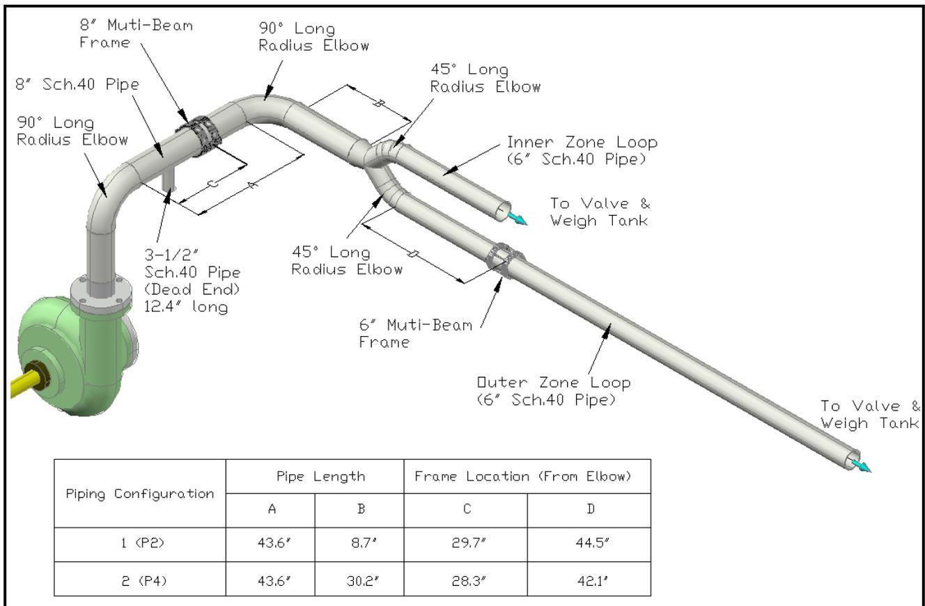
Figure 8 Laboratory piping configuration
