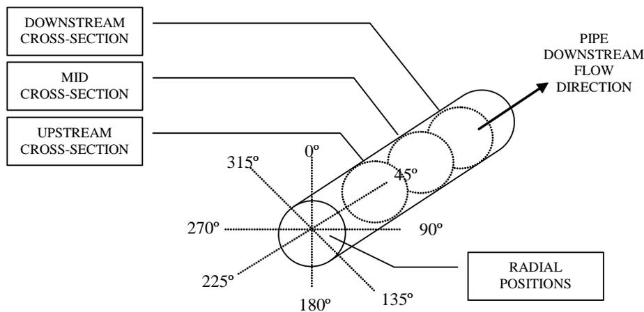
Figure 5 OD and thickness measurement scheme
