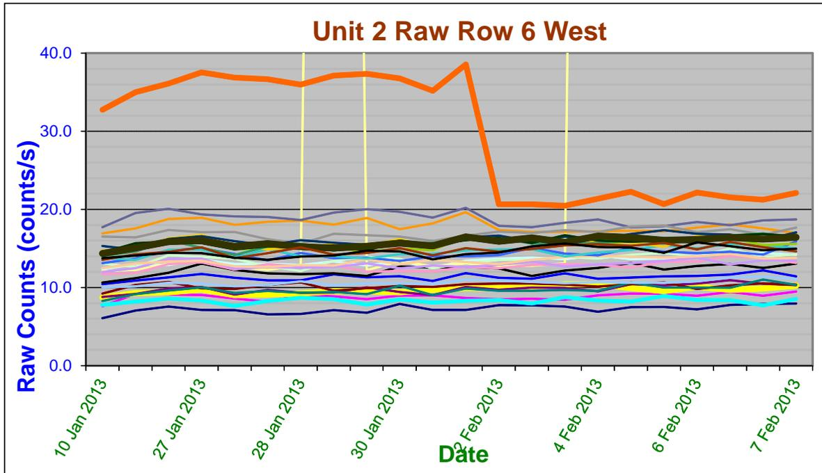
**Figure 7:** Raw counts from Unit 2 Row 6 west following unit Restart
