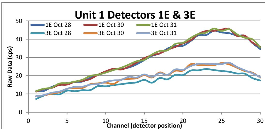
**Figure 1:** Raw data from two Unit 1 Detectors (1E and 3E) taken from three scans showing the typical shape of a detector's readings (with the lowest points between positions 1 and 8 and the highest readings between positions 20 and 28 [2]).
