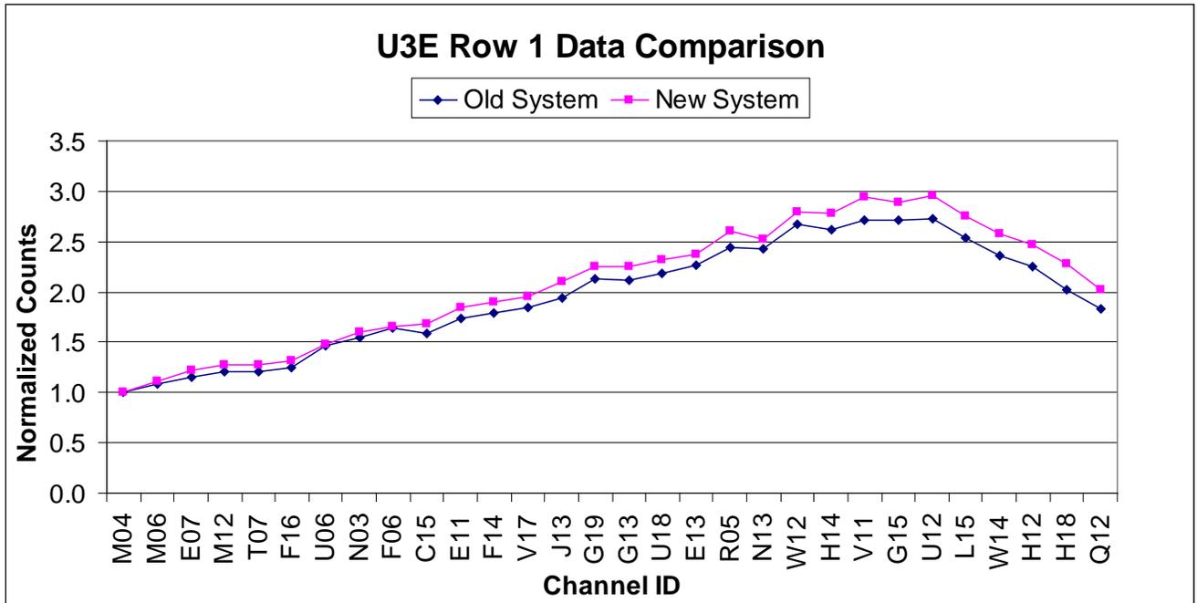
**Figure 5:** Comparison of data gathered from the new and old DN systems for Unit 3.
