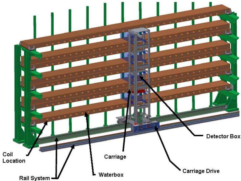
**Figure 4:** General arrangement of DN carriage, detector boxes and coils surrounded by a waterbox [4].
