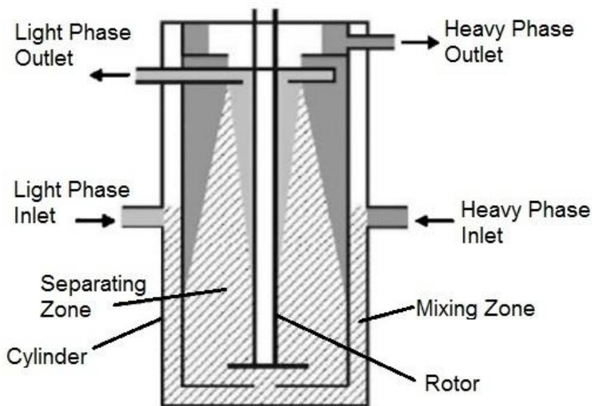
**Figure 2 Schematic of a Centrifugal Contactor [8]**
