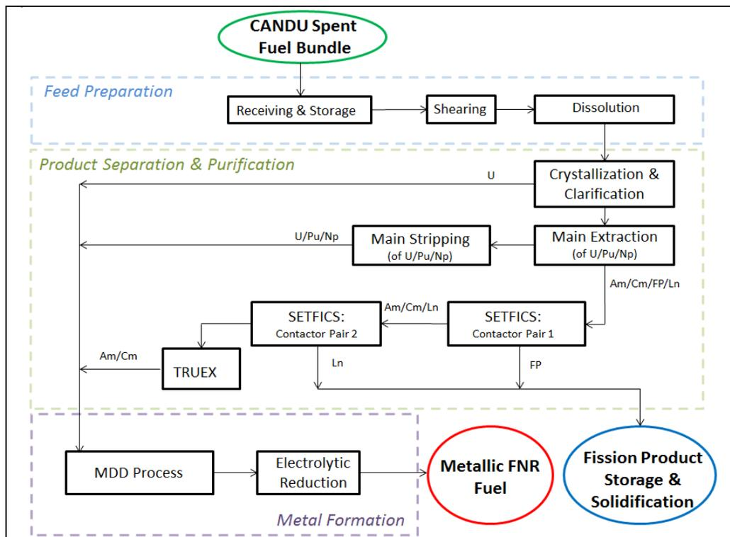
**Figure 1: Overall Process Block Diagram for the Modified PUREX Process**
