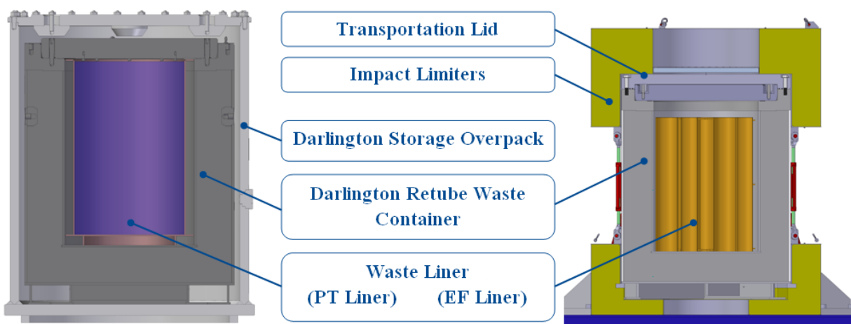
Figure 2: Darlington RWC System – Major Components
