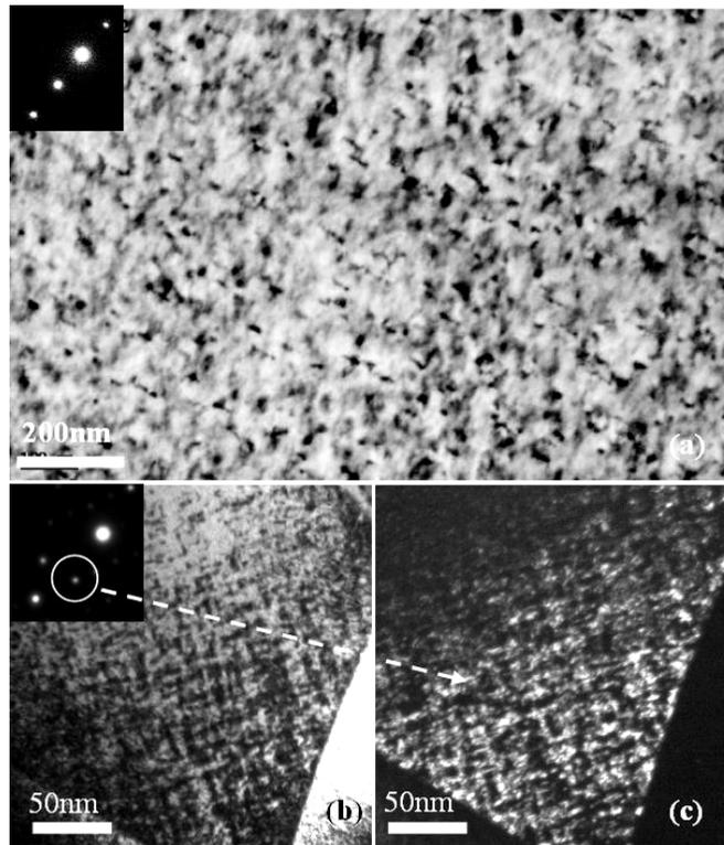
Fig.5. Major observations at 100°C after irradiations to 10 dpa. (a) shows the uniform distribution of c-loops in  $\alpha$ -phase. Length of the segments is decreased as compared to 400°C.  $g=0002$ ,  $B\sim[11\bar{2}0]$  (b). BF micrograph showing the presence of  $\omega$ -phase arranged in rectangular patterns, which is visible in form of thin Plates when imaged by selecting the  $\omega$ -reflection (encircled) in SADP,  $g=\bar{2}11$   $B\sim[011]$  (c).
