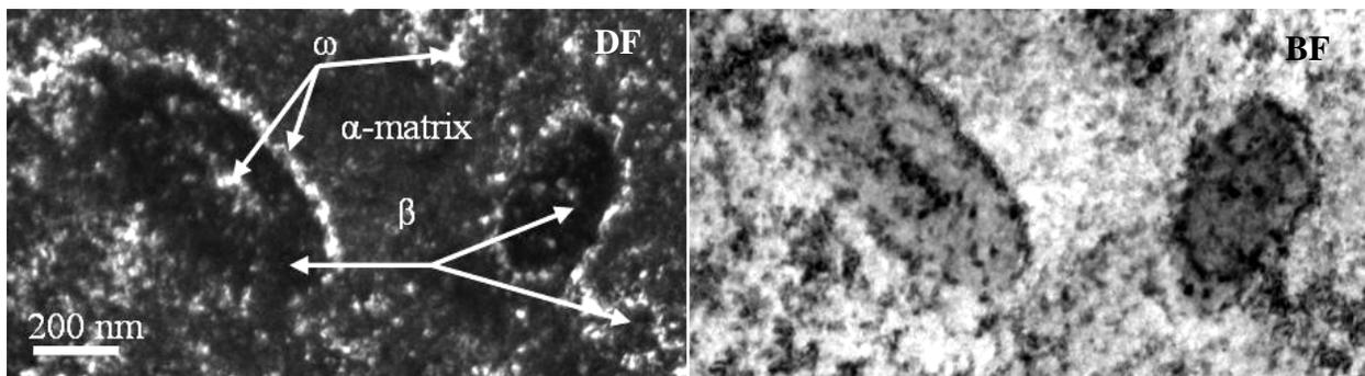
Fig. 3. showing the precipitation of growth of  $\omega$ -phase in the small  $\beta$ -phase islands present in  $\alpha$ -matrix. Cube shape  $\omega$ -phase precipitates and grow preferentially at the  $\alpha/\beta$  boundary. Some particles are present in the centre of  $\beta$ -phase islands.
