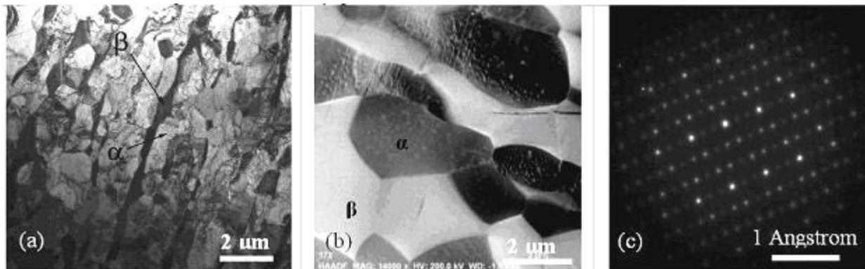
Fig. 1. (a) BF micrograph showing as received material microstructure, (b) HADF z-contrast image showing microstructure of heat treated material. (c). SAD pattern showing extra reflections from  $\omega$ - phase.
