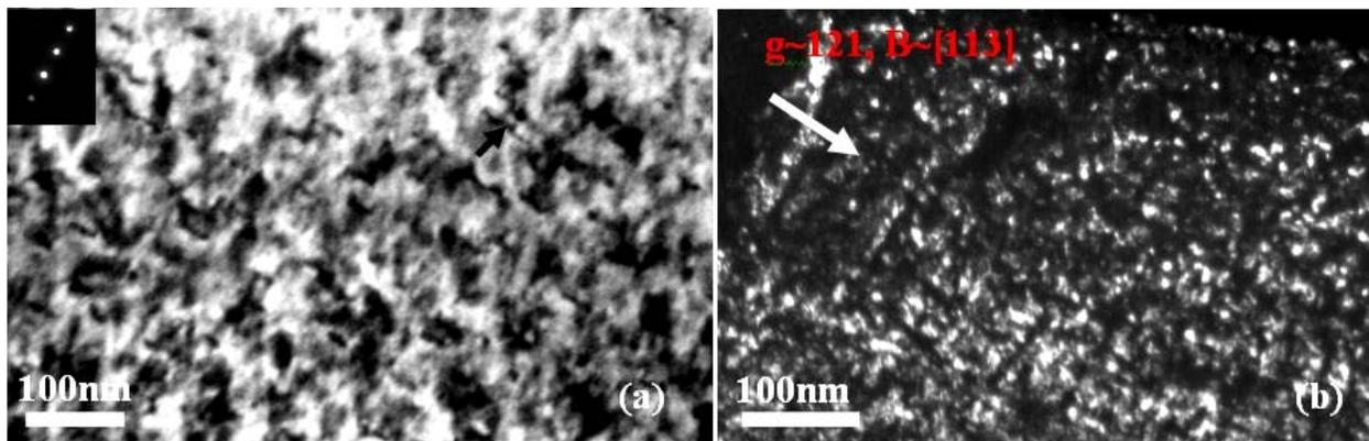
Fig. 4. (a). shows the presence of c-loops in form of thin short segments (arrowed) in  $\alpha$ -phase at 300°C at a dose level of 10 dpa,  $g=0002$   $B\sim[11\bar{2}0]$  (b). Cube shape  $\omega$ -phase precipitates similar to those observed at 400°C.
