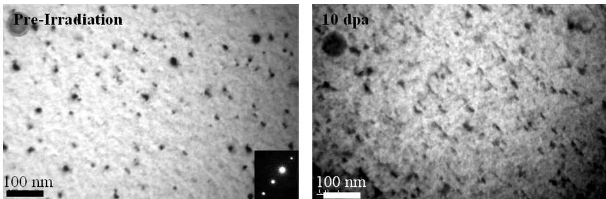
Fig. 2. Formation of c- loops in  $\alpha$ -phase; c-loops nucleate and grow in the vicinity of SPP at 400°C and 10 dpa. SPP disappear as the loops grow.  $g=0002$ ,  $B\sim[11\bar{2}0]$ .
