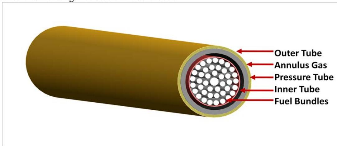
**Figure 1: Re-Entrant fuel Channel**
