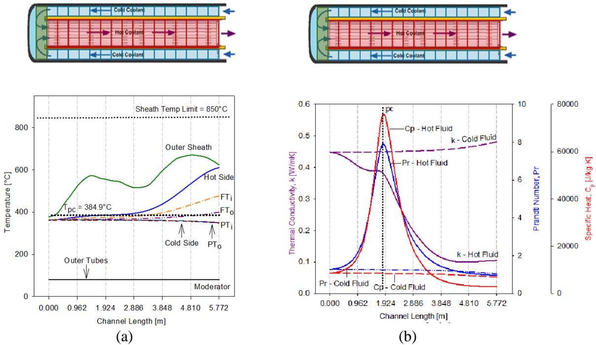
**Figure 3: (a) Temperature profile along channel length; (b) Specific heat, thermal conductivity and Prandtl number profiles along fuel-channel**
