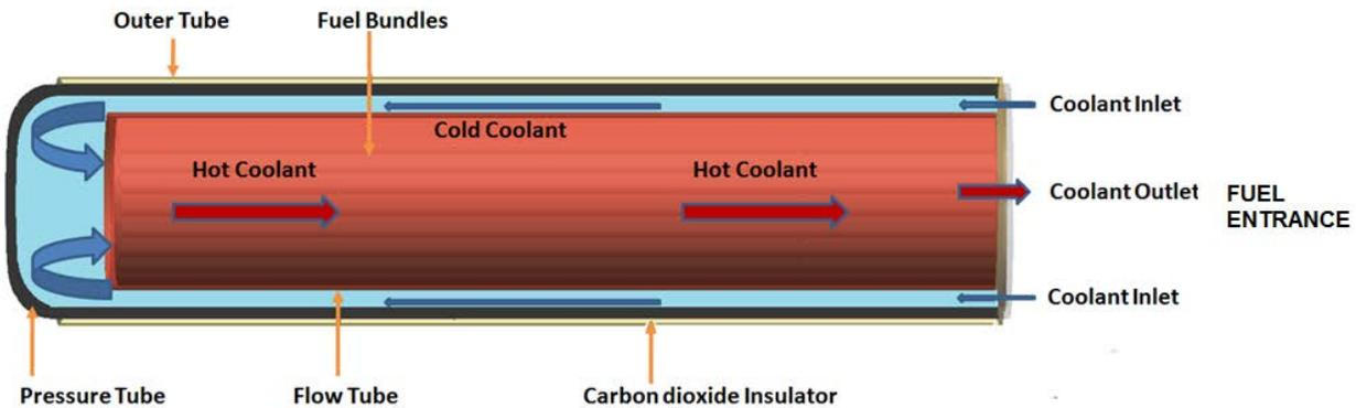
**Figure 2: Side view of the Re-Entrant fuel Channel**
