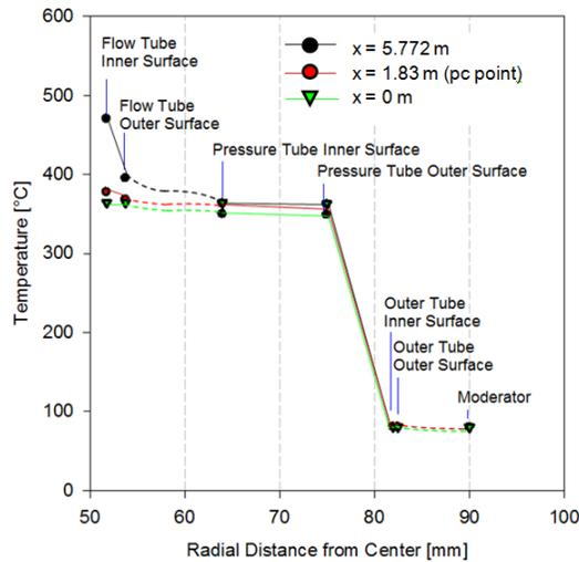
**Figure 4: Temperature gradients along radial distance from center for re-entrant channel.**
