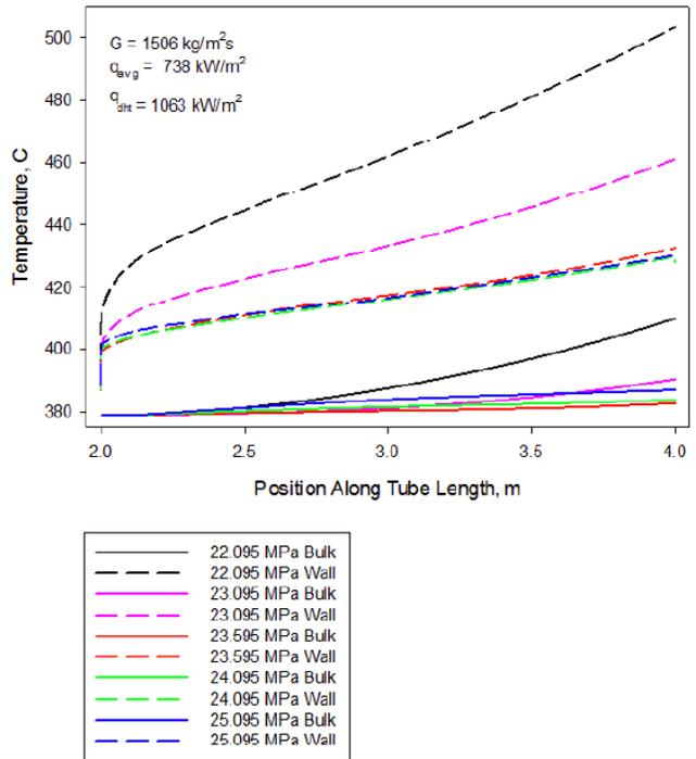
Figure 2: Bulk and Wall Temperature Distributions with Various Pressures
