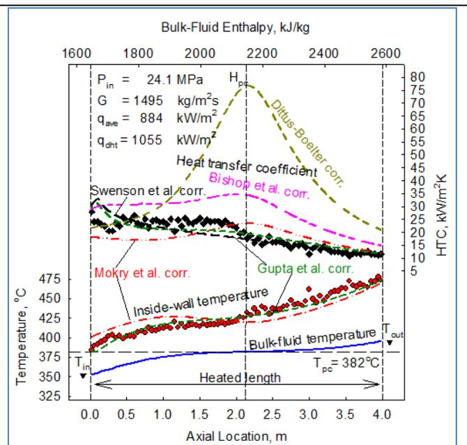
Figure 4: Comparison of *HTC* values calculated through various correlations with experimental data of 4-m circular vertical bare tube ( $D=10\text{mm}$ ):  $P_{in} \sim 24\text{ MPa}$  and  $G \sim 1500\text{ kg/m}^2\text{s}$ .
