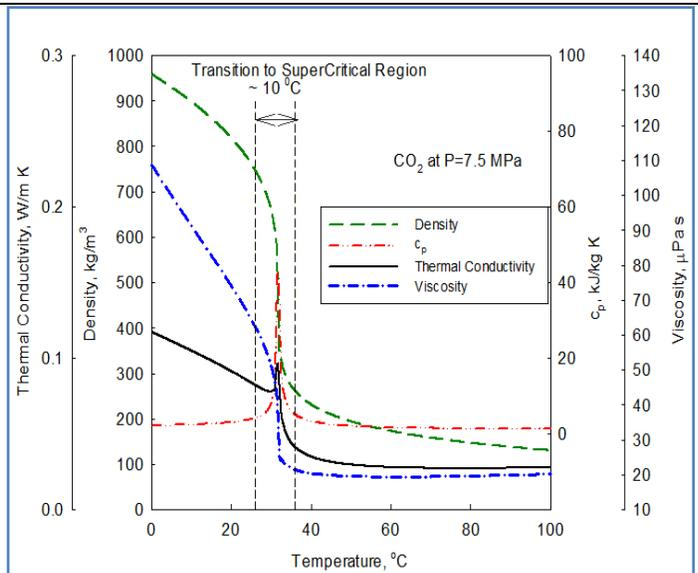
Figure 2: Thermophysical properties profiles of supercritical CO<sub>2</sub> as function of temperature at 7.5 MPa
