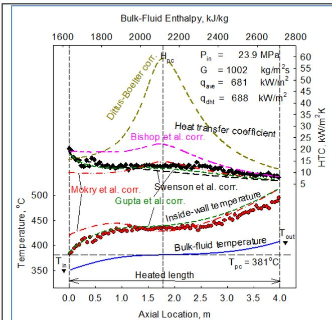
Figure 3: Comparison of *HTC* values calculated through various correlations with experimental data<sup>1</sup> of 4-m circular vertical bare tube ( $D=10\text{mm}$ ):  $P_{in} \sim 24\text{ MPa}$  and  $G \sim 1000\text{ kg/m}^2\text{s}$ .
