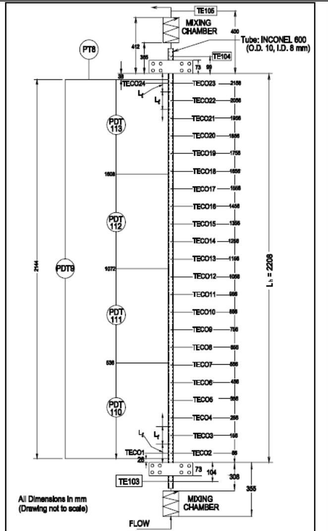
**Figure 5: Test Section of MR-1 Loop [1]**
