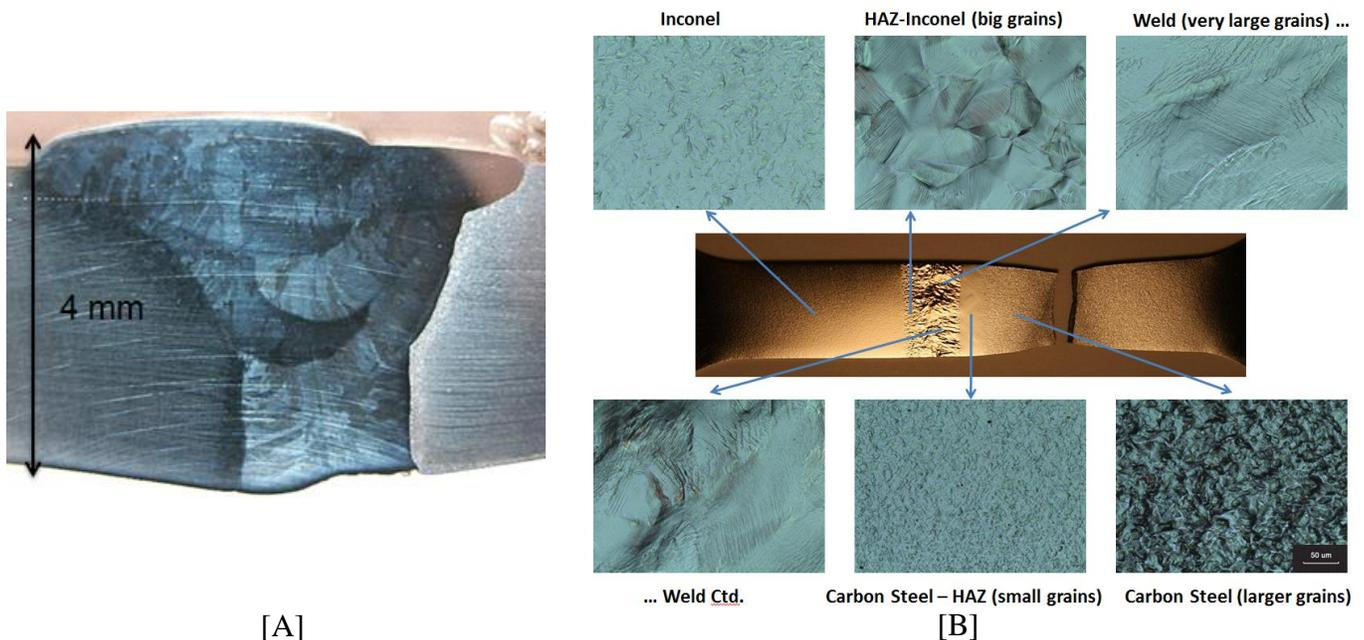
Figure 2 [A] Whole Weld Cross-Section Polished and Etched (Left to Right: Inconel 600, Inconel 82 Weld Filler, Carbon Steel (Grade 106 B)) [B] Microstructure after tensile test (Scale in bottom right valid for all images)
