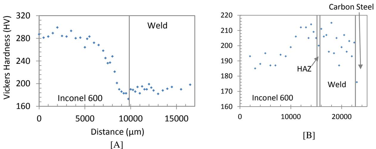
Figure 1 [A] Hardness Test 0.3 mm from the Outer Diameter [B] Hardness Test 7 mm from the Outer Diameter ( $\approx 1$  mm from ID)
