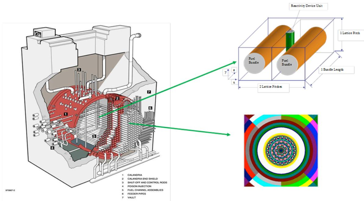
Figure 2 Illustration of RFSP Modelling of a CANDU Core
