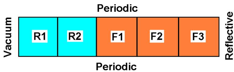
Figure 4 Schematic representation of the planar-type core-reflector interface
