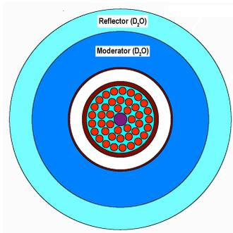
Figure 3 Super-cell model used for the calculation of reflector properties
