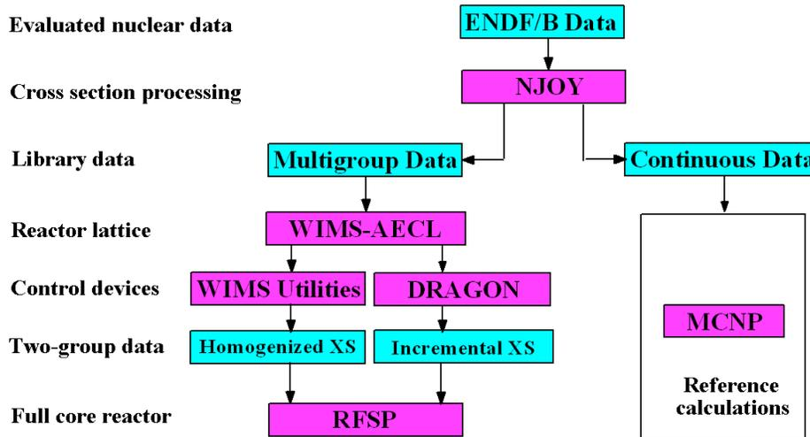
Figure 1 The 3-stage scheme of deterministic neutronics calculations as a part of AECL’s reactor physics computational scheme
