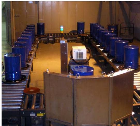
Figure 5 Stationary system for RW characterisation with a conveyer for 25 drums at Radon Moscow (Russia)
