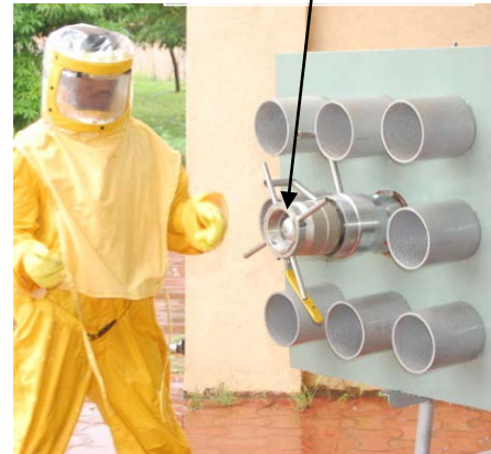
Leakage arrested completely
