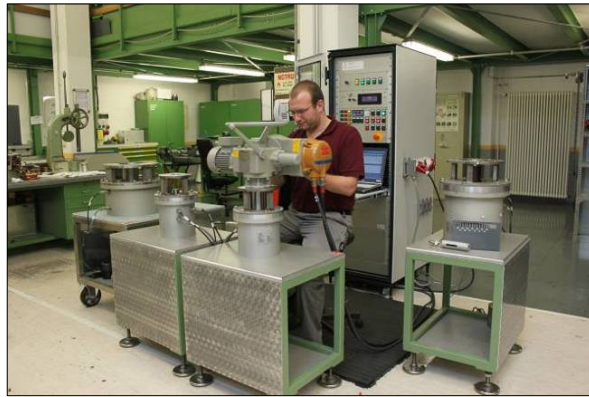
Figure 7 ADAM® system with MDP test benches and control panel in a workshop
