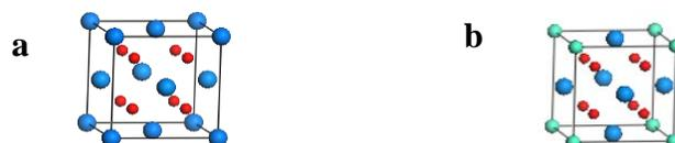
Figure 1 Lattice structure of pure urania and thoria (a) and mixed fuel (b) with Plutonium (25% atomic substitution of U). Uranium, thorium, plutonium and oxygen atoms are marked as spheres, with the radius ranging from the largest for U and Th atoms to the smallest for O atoms.
