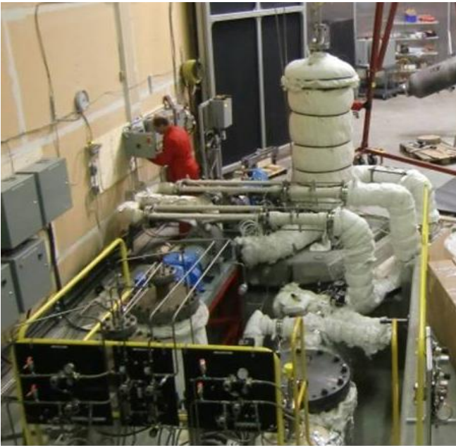
Figure 2: (Top) Photograph of the Mini-Sphere with piston housings installed. (Left) Photograph of the Pb pumping system including Pb pumps, melt vessel, de-bubbling vessels, and a section of Pb piping. (Right) Schematic of the 14-piston liquid Pb Mini-Sphere connected to the Pb pumping system.
