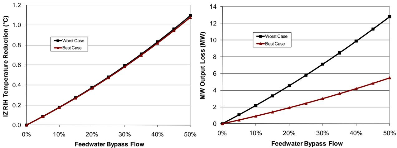
**Figure 7&8 RIHT Drop & Gross Electrical Output Loss due to FW Bypass Flow**
