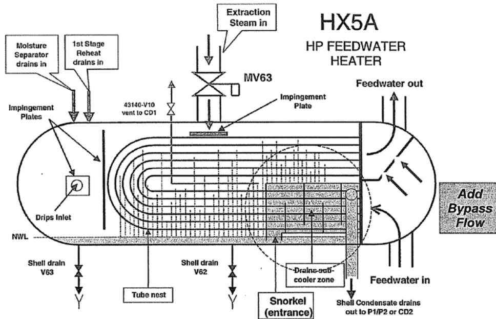
Figure 6: FW bypass flow of HP FW heater tube bundle
