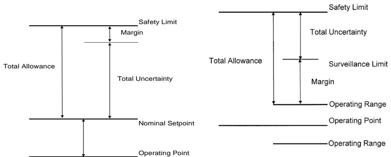
**Figure 1&2: SOE Compliance for an Actuation (L) & Indication (R) Parameter**
