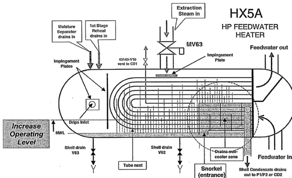
**Figure 9: Partial flooding of HP FW heater shell side**
