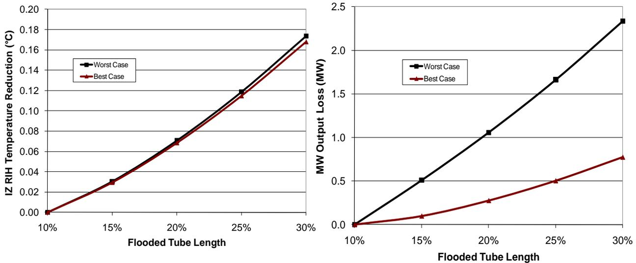
**Figure 10&11: RIHT Drop & Electrical Output Loss due to Partial Flooding**
