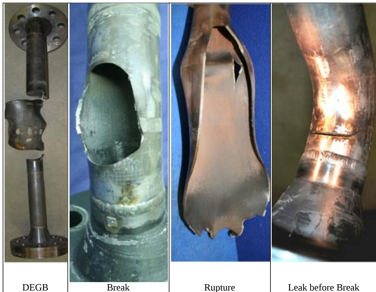
Figure 10: Mode of Failure of Specimens with Severe Local Thinning Tested under FBTP-3
