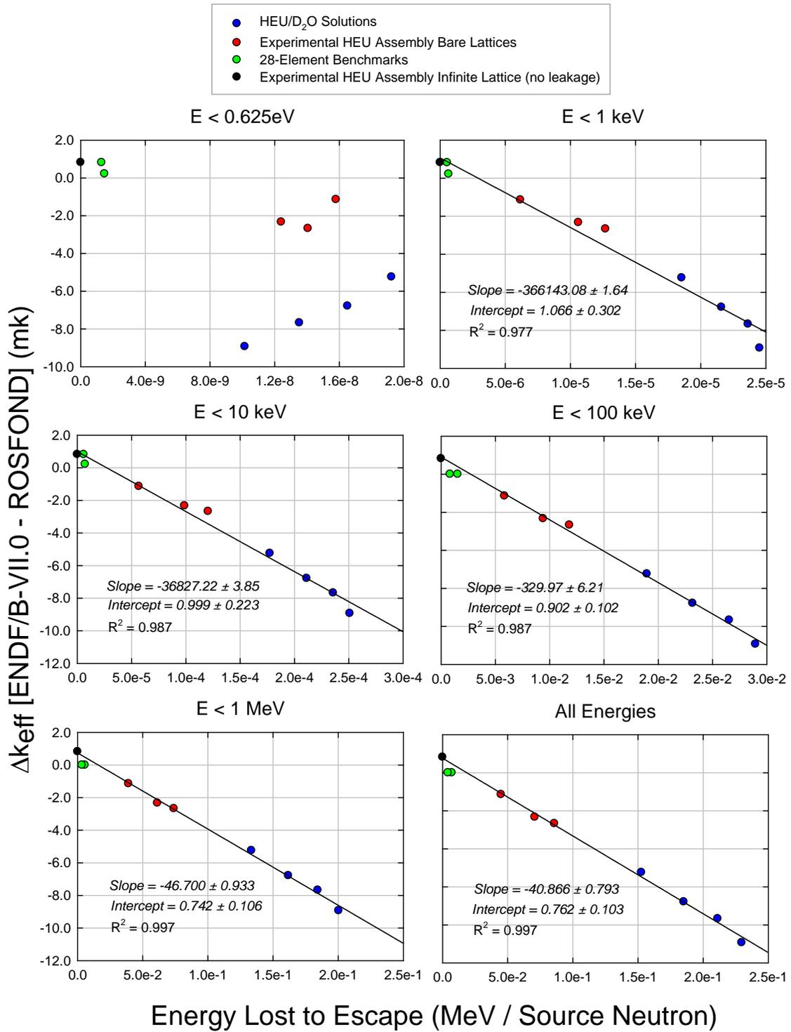
Figure 5 Sensitivity of Core to Deuterium Scattering Data Evaluation as a Function of Energy lost to Leakage for Several Neutron Energy Ranges
