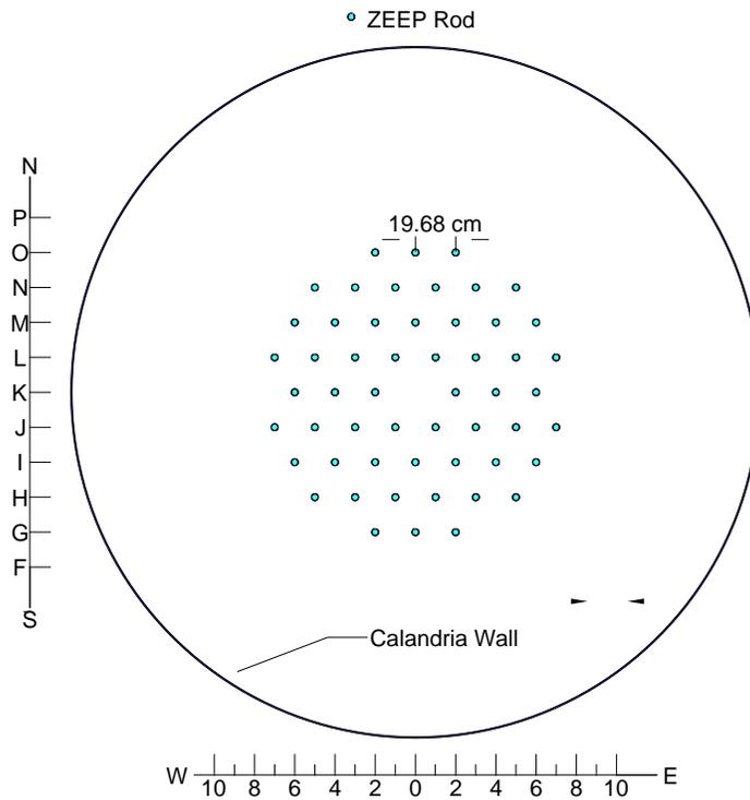
Figure 3 Plan View of 54 ZEEP Rod Reference Lattice (K0 Empty)
