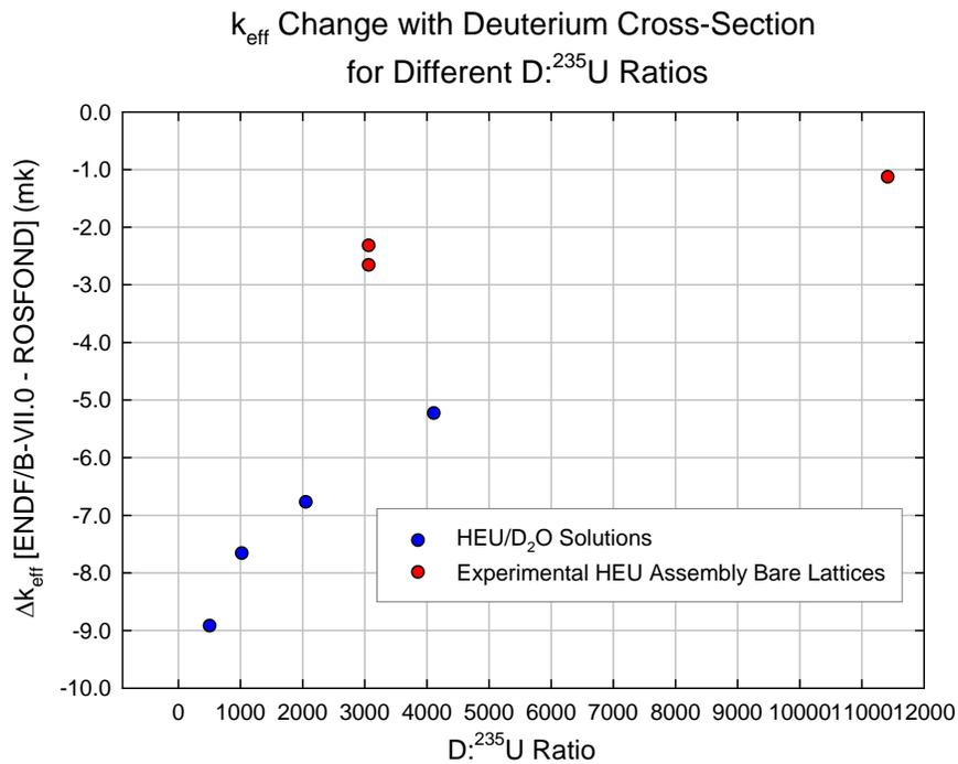
Figure 4 Sensitivity of Core to Deuterium Scattering Data Evaluation as a Function of D:<sup>235</sup>U Ratio
