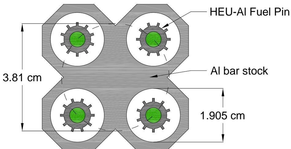
Figure 2 Cross section of Experimental HEU Assembly Used for ZED-2 Experiments
