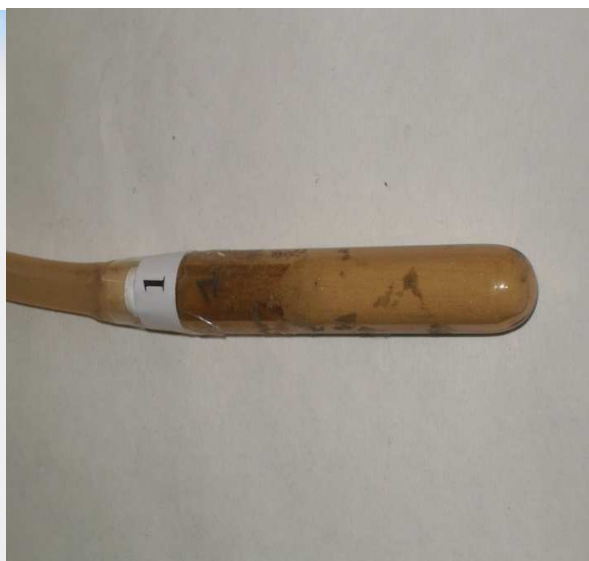
Figure 6. Irradiation test of N960 to determine gas generation
