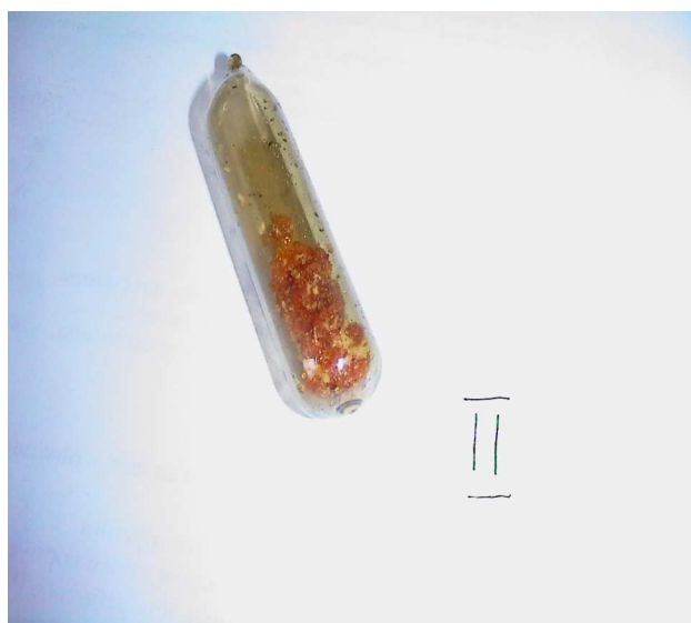
Figure 5. Irradiation experiment on nitric organic solution
