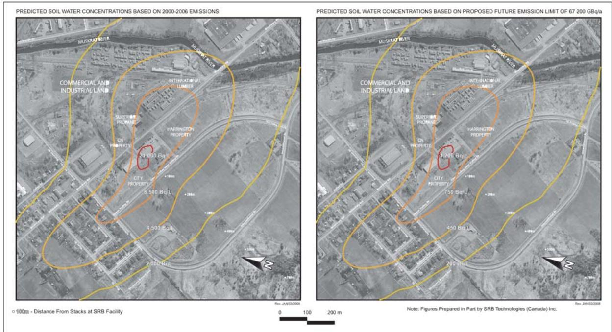
**Figure 8. Predicted Soil Water Contours Based on Average 2000-2006 Emissions and Based on the New Emission Limit**
