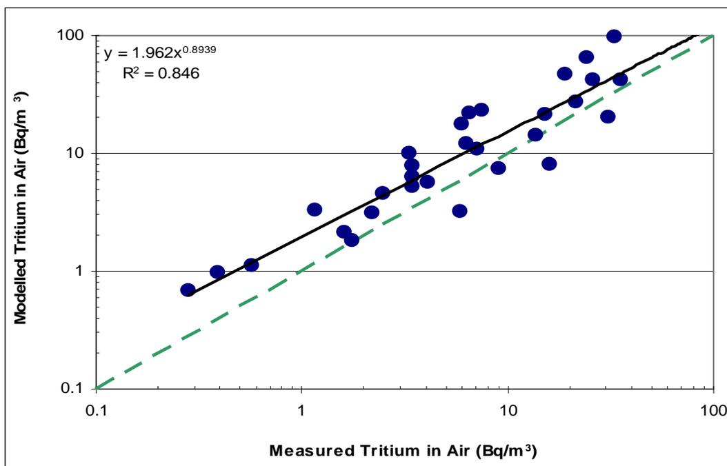
Figure 6. Modeled vs Measured Tritium in Air ( 0-3 km)
